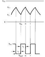
Note: The equations assume  $t_1+t_2>>t_{pd0}+t_{pd1}$
