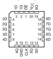
OE does not affect the internal operations of the flip-flops. Old data can be retained or new data can be entered while the outputs are in the high-impedance state.
