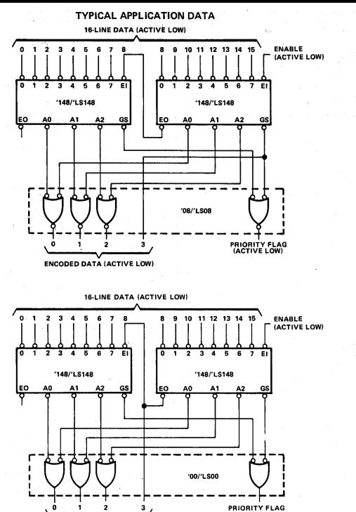
Since the '147/'LS147 and '148/'LS148 are combinational logic circuits, wrong addresses can appear during input transients. Moreover, for the '148/'LS148 a change from high to low at input El can cause a transient low on the GS output when all inputs are high. This must be considered when strobing the outputs.
