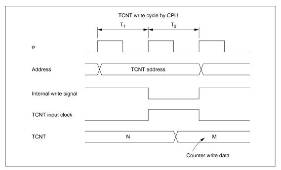
Figure 10.11 Contention between TCNT Write and Increment
