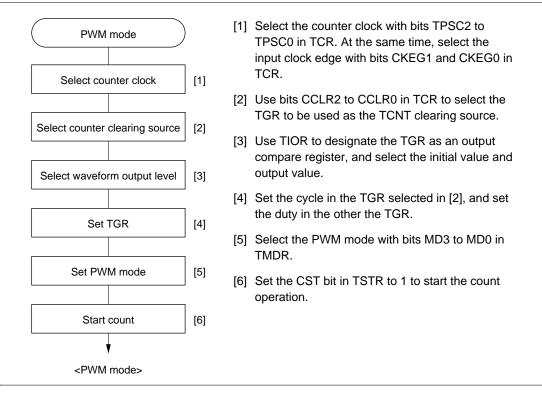
Figure 9.24 Example of PWM Mode Setting Procedure
