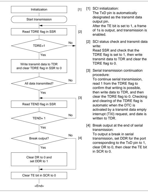
Figure 12.5 Sample Serial Transmission Flowchart
