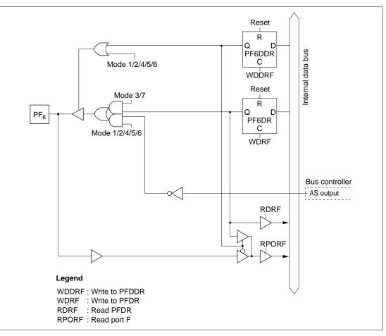
Figure C.10 (g) Port F Block Diagram (Pin PF<sub>6</sub>)
