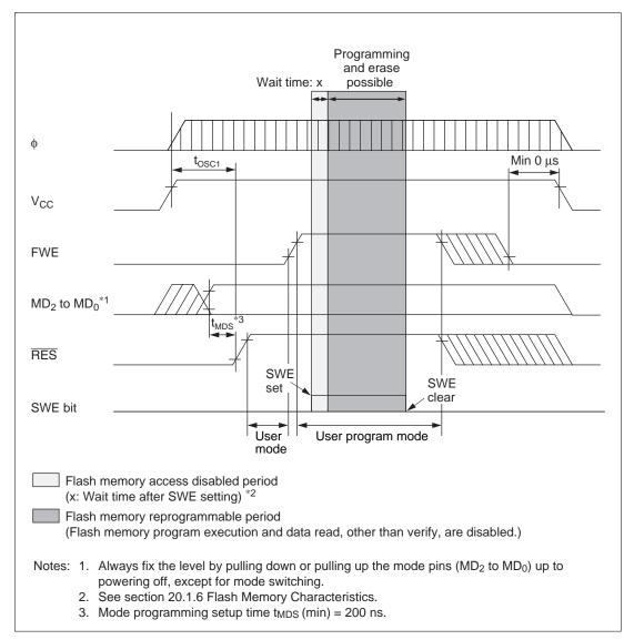
Figure 17.37 Powering On/Off Timing (User Program Mode)
