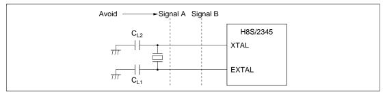
Figure 18.4 Example of Incorrect Board Design
