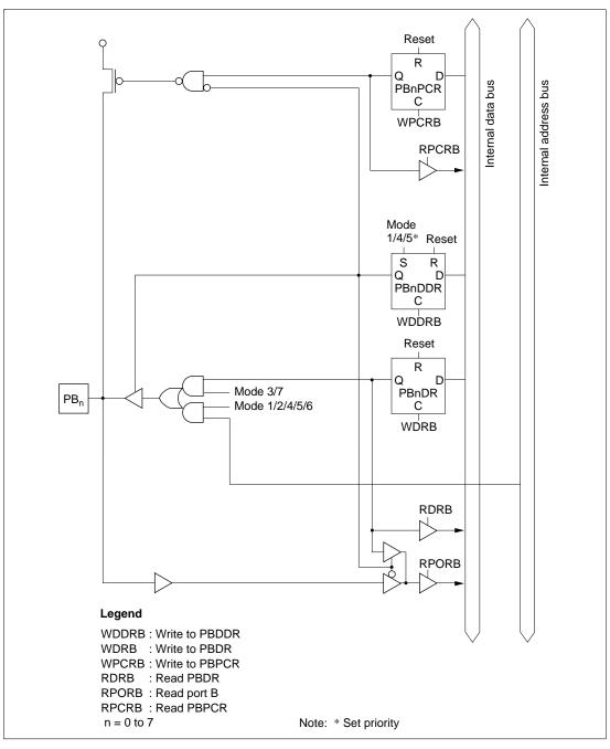
Figure C.6 Port B Block Diagram (Pin PB<sub>n</sub>)
