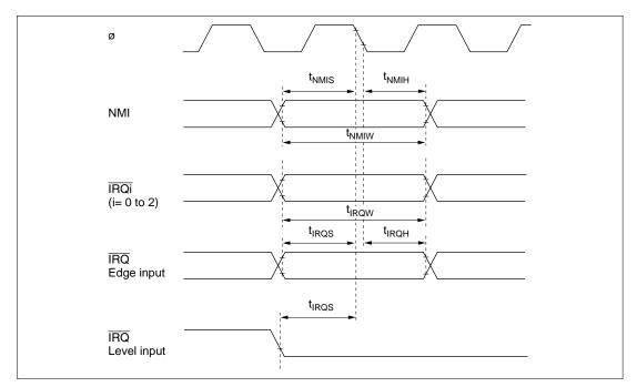
Figure 20.10 Interrupt Input Timing
