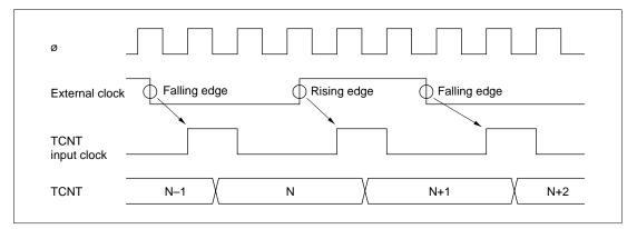
Figure 9.35 Count Timing in External Clock Operation
