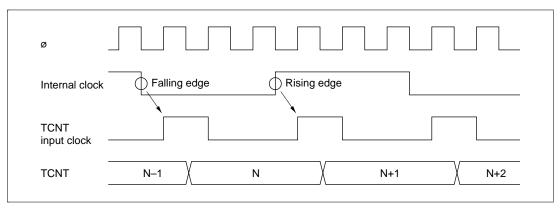
Figure 9.34 Count Timing in Internal Clock Operation
