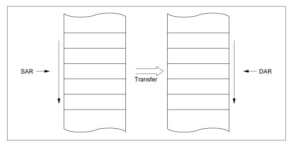
Figure 7.6 Memory Mapping in Normal Mode
