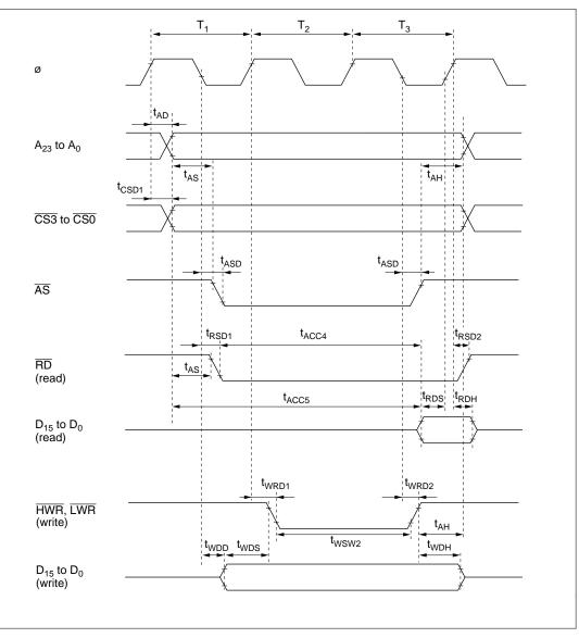
Figure 20.12 Basic Bus Timing (Three-State Access)
