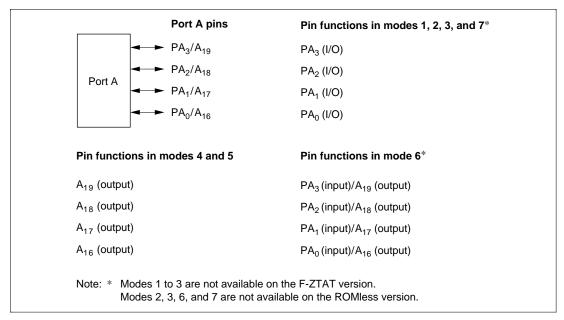
Figure 8.5 Port A Pin Functions
