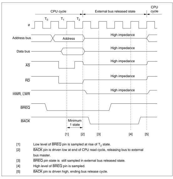
Figure 6.19 Bus-Released State Transition Timing
