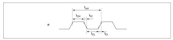
Figure 20.7 System Clock Timing
