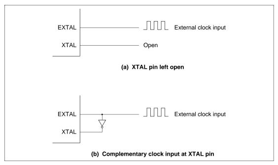
Figure 18.5 External Clock Input (Examples)
