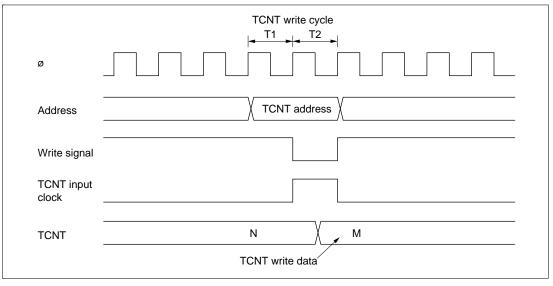
Figure 9.50 Contention between TCNT Write and Increment Operations
