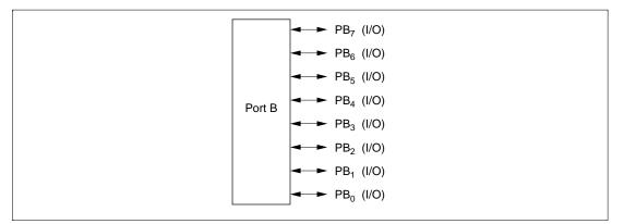
Figure 8.12 Port B Pin Functions (Modes 3 and 7)\*
