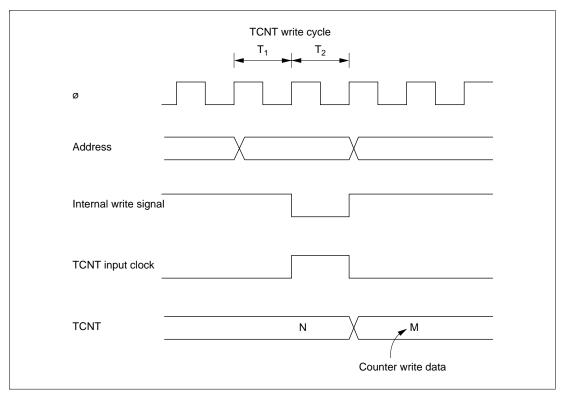
Figure 11.8 Contention between TCNT Write and Increment
