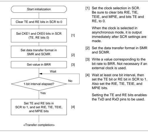
Figure 12.4 Sample SCI Initialization Flowchart
