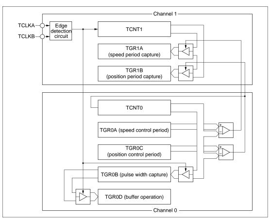
Figure 9.33 Phase Counting Mode Application Example
