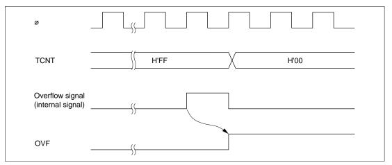
Figure 11.6 Timing of Setting of OVF
