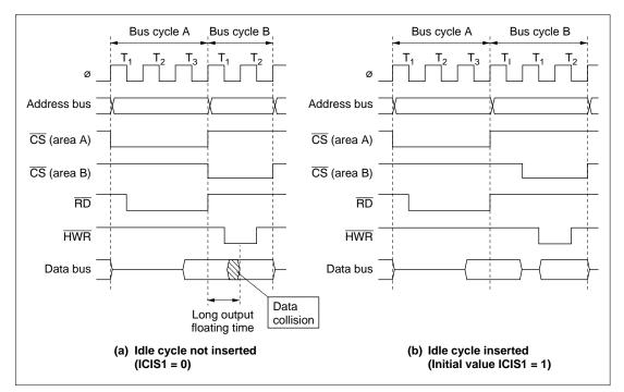
Figure 6.17 Example of Idle Cycle Operation (2)
