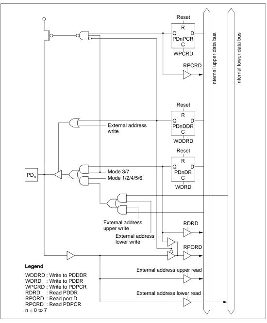
Figure C.8 Port D Block Diagram (Pin PD<sub>n</sub>)
