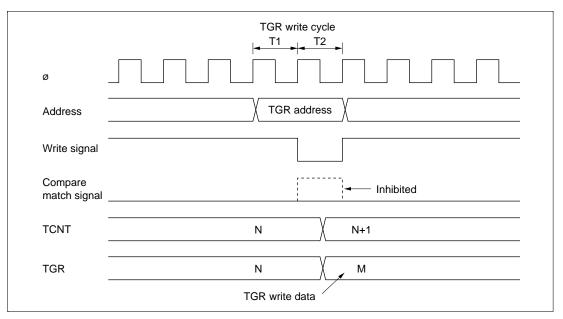
Figure 9.51 Contention between TGR Write and Compare Match
