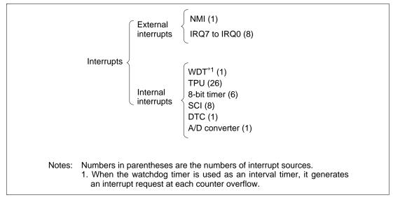
Figure 4.4 Interrupt Sources and Number of Interrupts
