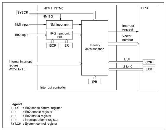
A block diagram of the interrupt controller is shown in Figure 5.1.
