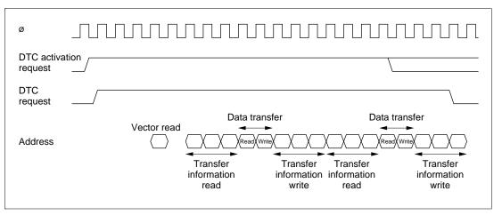
Figure 7.12 DTC Operation Timing (Example of Chain Transfer)
