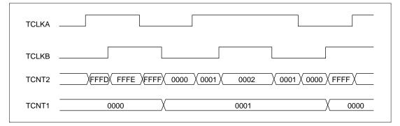
Figure 9.23 Example of Cascaded Operation (2)
