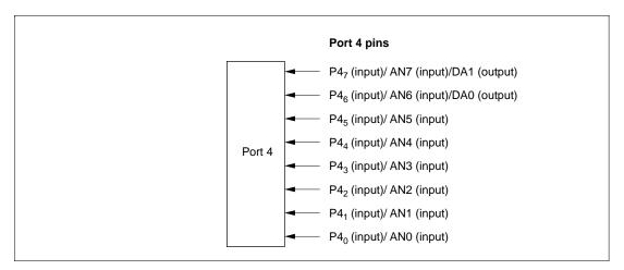
Figure 8.4 Port 4 Pin Functions
