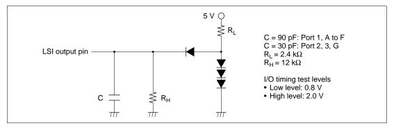
Figure 20.6 Output Load Circuit
