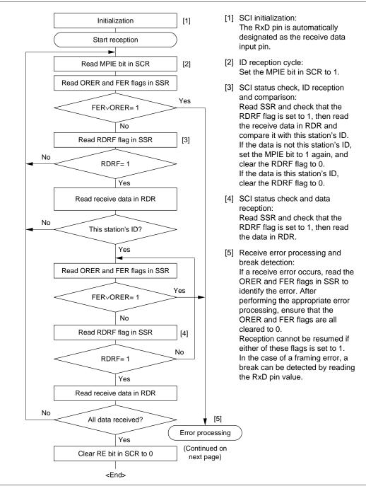
Figure 12.12 Sample Multiprocessor Serial Reception Flowchart
