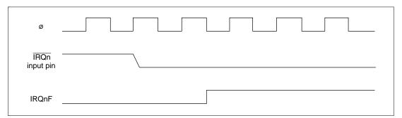
Figure 5.3 Timing of Setting IRQnF
