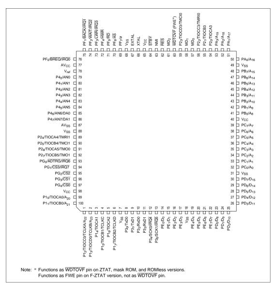
Figures 1.2 and 1.3 show the pin arrangement of the H8S/2345 Series.
