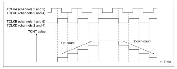
Figure 9.32 Example of Phase Counting Mode 4 Operation
