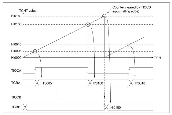
Figure 9.13 Example of Input Capture Operation
