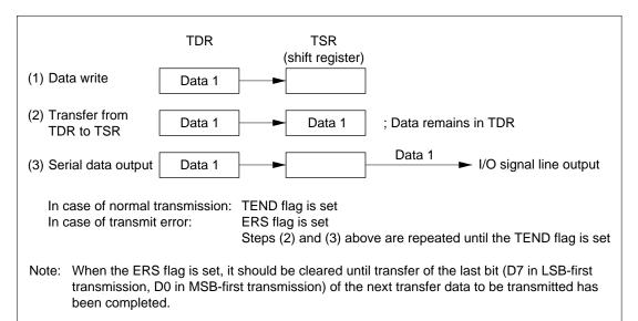
Figure 13.5 Relation Between Transmit Operation and Internal Registers
