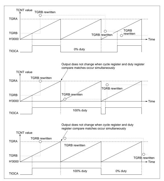
Figure 9.27 shows examples of PWM waveform output with 0% duty and 100% duty in PWM mode.
