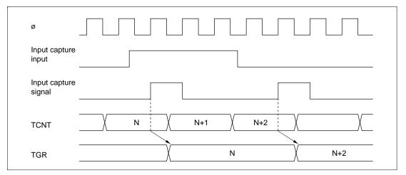
Figure 9.37 Input Capture Input Signal Timing
