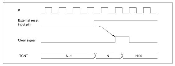
Figure 10.7 Timing of External Reset
