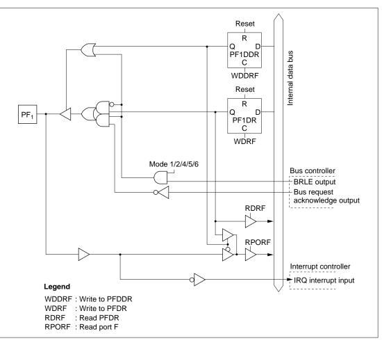
Figure C.10 (b) Port F Block Diagram (Pin PF<sub>1</sub>)
