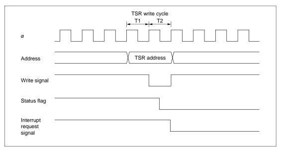
Figure 9.46 Timing for Status Flag Clearing by CPU
