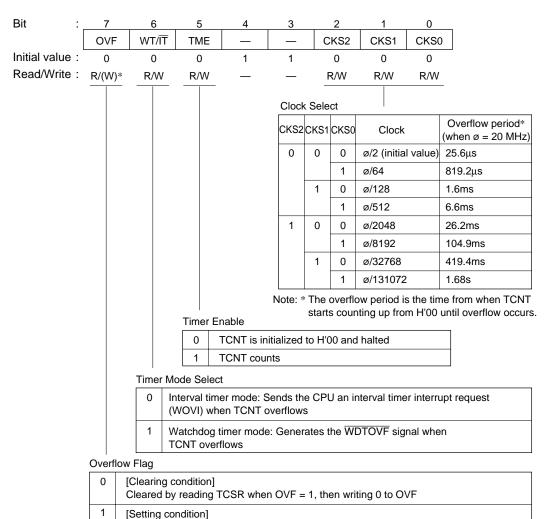
Set when TCNT overflows from H'FF to H'00 in interval timer mode
