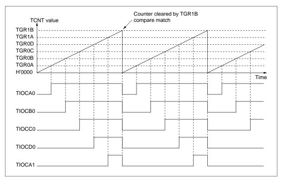
Figure 9.26 Example of PWM Mode Operation (2)
