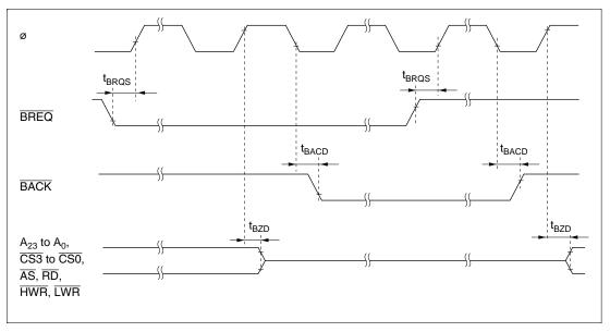
Figure 20.16 External Bus Release Timing
