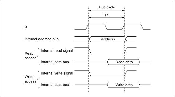
Figure 2.17 On-Chip Memory Access Cycle
