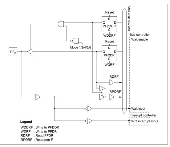
Figure C.10 (c) Port F Block Diagram (Pin PF<sub>2</sub>)
