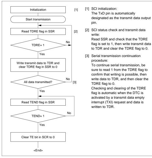
Figure 12.16 Sample Serial Transmission Flowchart
