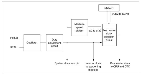
Figure 18.1 Block Diagram of Clock Pulse Generator
