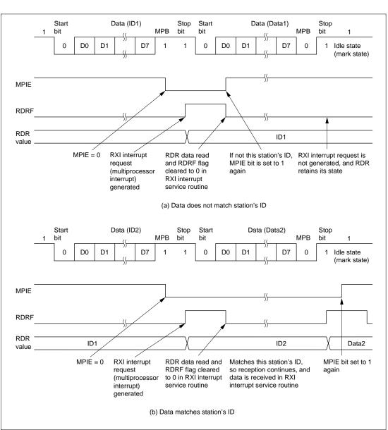
Figure 12.13 shows an example of SCI operation for multiprocessor format reception.
