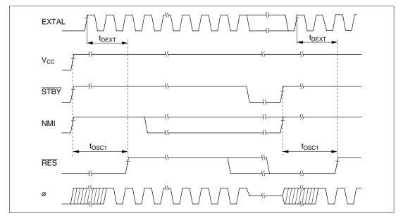
Figure 20.8 Oscillator Settling Timing
