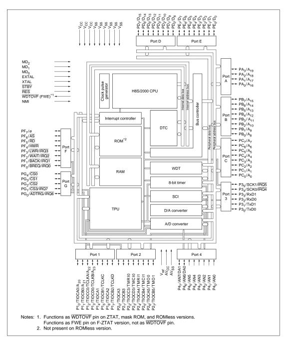
Figure 1.1 Block Diagram
