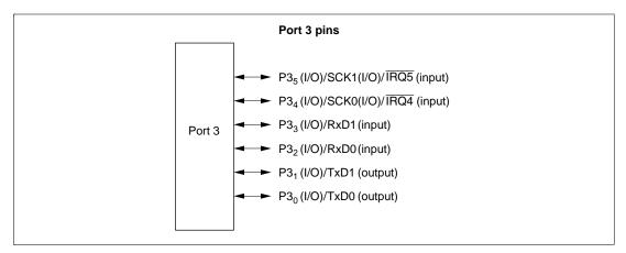
Figure 8.3 Port 3 Pin Functions
