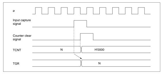
Figure 9.39 Counter Clear Timing (Input Capture)
