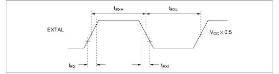
Figure 18.6 External Clock Input Timing
