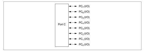
Figure 8.16 Port C Pin Functions (Modes 3 and 7)\*
