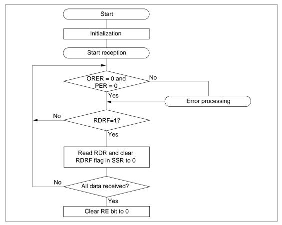
Figure 13.7 Example of Reception Processing Flow
