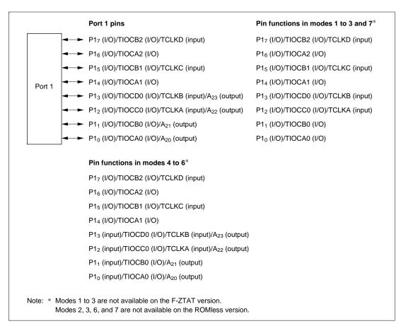
Figure 8.1 Port 1 Pin Functions
