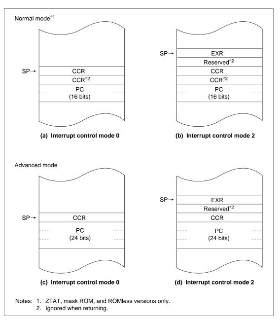
Figure 2.16 Stack Structure after Exception Handling (Examples)
