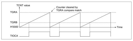
Figure 9.25 Example of PWM Mode Operation (1)
