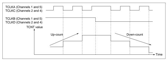
Figure 9.30 Example of Phase Counting Mode 2 Operation
