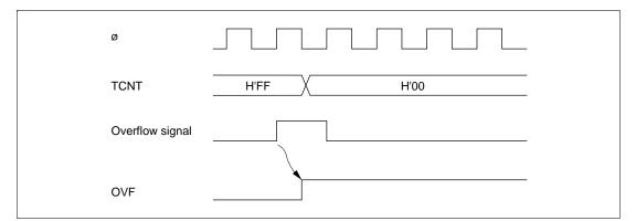
Figure 10.8 Timing of OVF Setting
