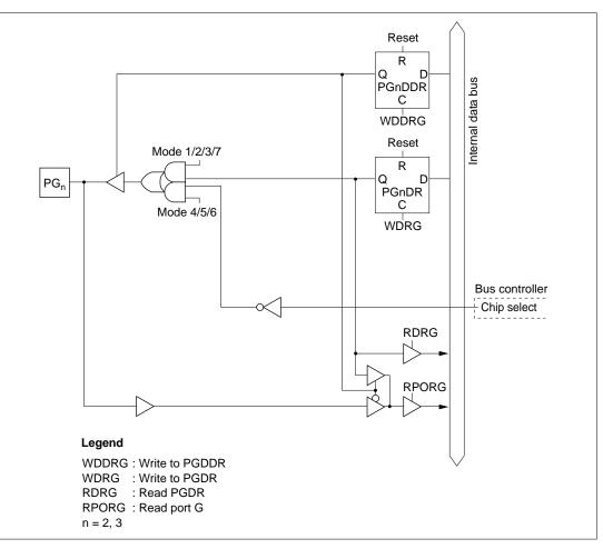
Figure C.11 (c) Port G Block Diagram (Pins PG<sub>2</sub> and PG<sub>3</sub>)
