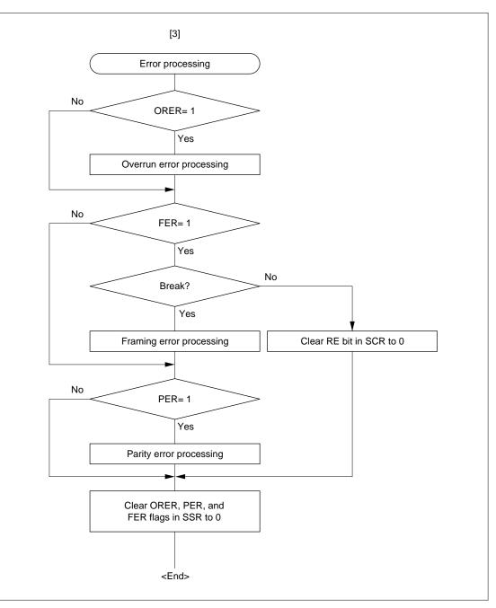
Figure 12.7 Sample Serial Reception Data Flowchart (cont)
