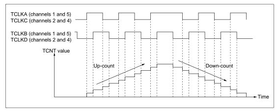
Figure 9.29 Example of Phase Counting Mode 1 Operation
