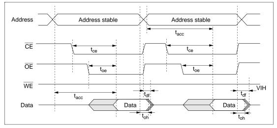
Figure 17.29 Timing Waveforms for **CE**/**OE** Clocked Read
