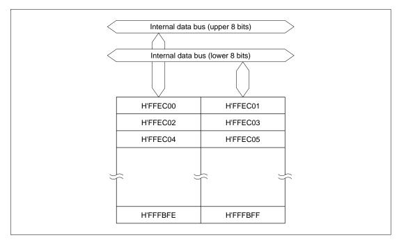
Figure 16.1 shows a block diagram of the on-chip RAM.
