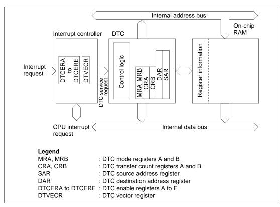
Figure 7.1 Block Diagram of DTC
