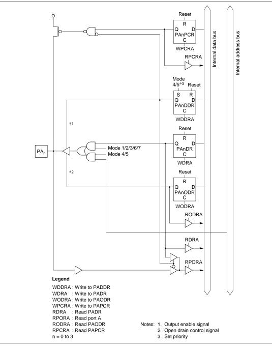
Figure C.5 Port A Block Diagram (Pins PA<sub>0</sub> to PA<sub>3</sub>)
