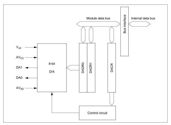
Figure 15.1 Block Diagram of D/A Converter
