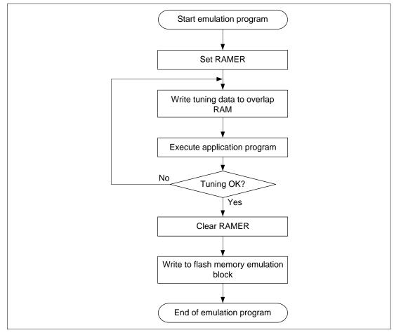
Figure 17.24 Flowchart for Flash Memory Emulation in RAM
