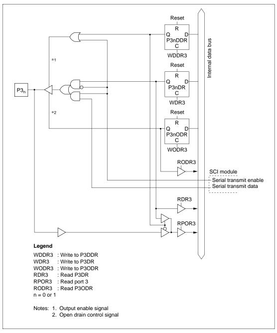
Figure C.3 (a) Port 3 Block Diagram (Pins P3<sub>0</sub> and P3<sub>1</sub>)
