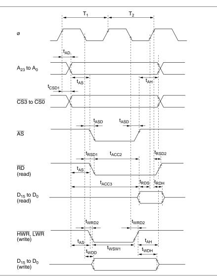
Figure 20.11 Basic Bus Timing (Two-State Access)
