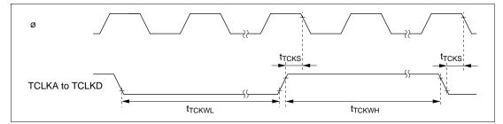
Figure 20.19 TPU Clock Input Timing
