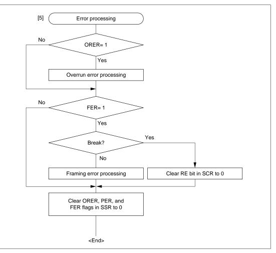
Figure 12.12 Sample Multiprocessor Serial Reception Flowchart (cont)
