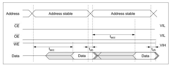
Figure 17.28 Timing Waveforms for **CE**/**OE** Enable State Read
