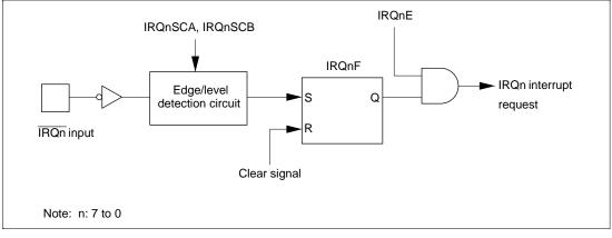
Figure 5.2 Block Diagram of Interrupts IRQ7 to IRQ0
