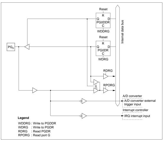
Figure C.11 (a) Port G Block Diagram (Pin PG<sub>0</sub>)
