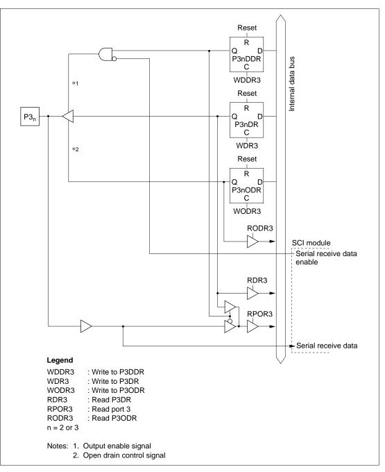
Figure C.3 (b) Port 3 Block Diagram (Pins P3<sub>2</sub> and P3<sub>3</sub>)
