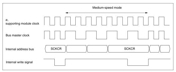
Figure 19.1 Medium-Speed Mode Transition and Clearance Timing
