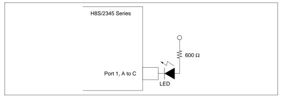
Figure 20.5 LED Drive Circuit (Example)
