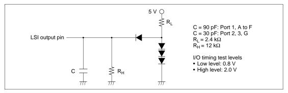
Figure 20.3 Output Load Circuit
