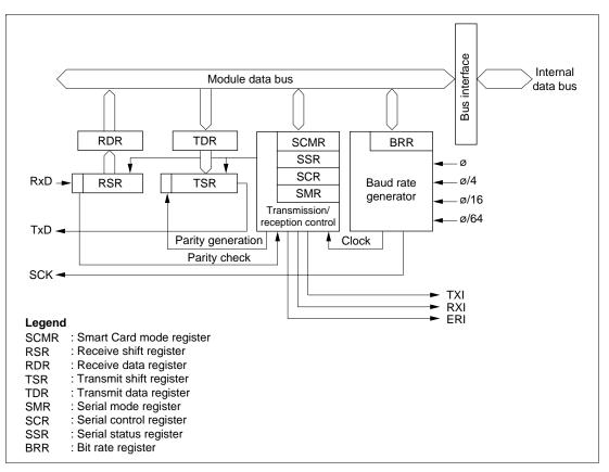
Figure 13.1 Block Diagram of Smart Card Interface
