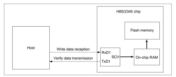
Figure 17.15 System Configuration in Boot Mode
