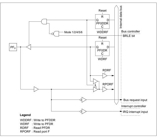
Figure C.10 (a) Port F Block Diagram (Pin PF<sub>0</sub>)
