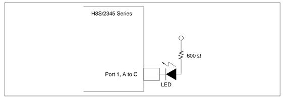
Figure 20.2 LED Drive Circuit (Example)
