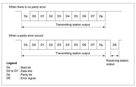
Figure 13.3 Smart Card Interface Data Format
