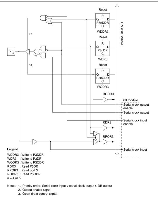
Figure C.3 (c) Port 3 Block Diagram (Pins P3<sub>4</sub> and P3<sub>5</sub>)
