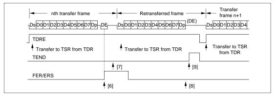
Figure 13.12 Retransfer Operation in SCI Transmit Mode
