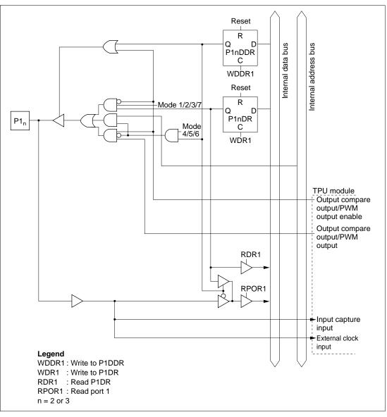
Figure C.1 (b) Port 1 Block Diagram (Pins P1<sub>2</sub> and P1<sub>3</sub>)
