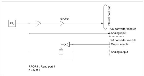
Figure C.4 (b) Port 4 Block Diagram (Pins P4<sub>6</sub> and P4<sub>7</sub>)
