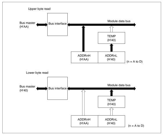
Figure 14.2 ADDR Access Operation (Reading H'AA40)
