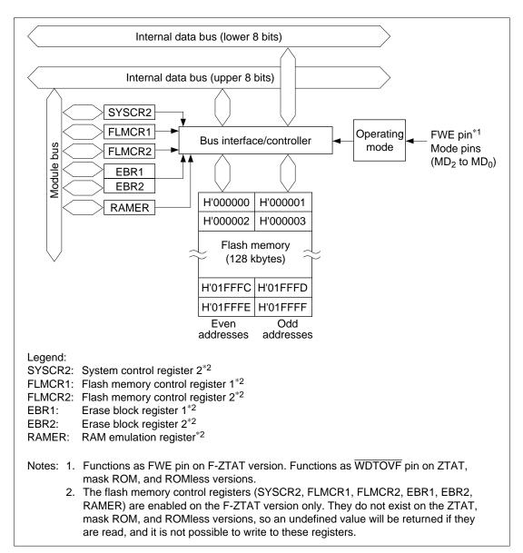
Figure 17.7 Block Diagram of Flash Memory
