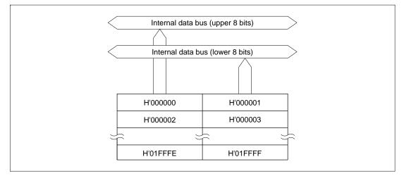
Figure 17.1 Block Diagram of ROM (H8S/2345)
