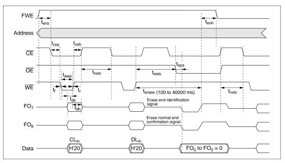
Figure 17.32 Auto-Erase Mode Timing Waveforms
