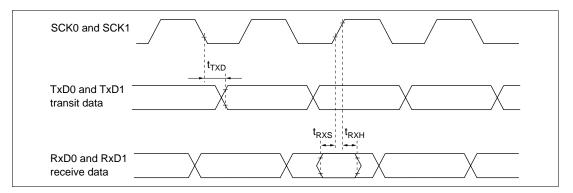
Figure 20.25 SCI Input/Output Timing (Clock Synchronous Mode)
