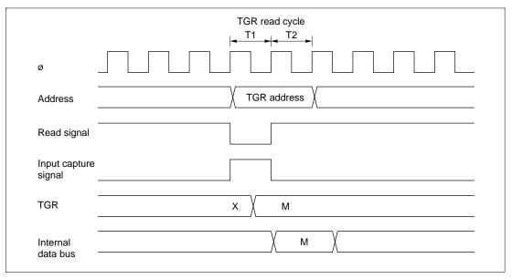
Figure 9.53 Contention between TGR Read and Input Capture
