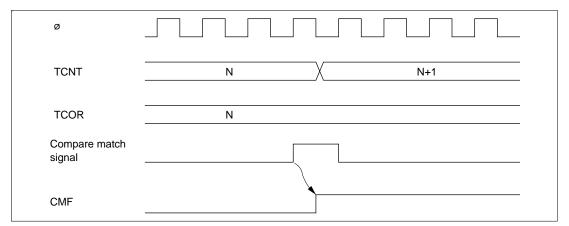
Figure 10.4 Timing of CMF Setting
