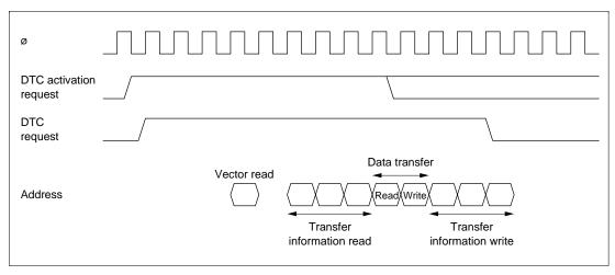
Figure 7.10 DTC Operation Timing (Example in Normal Mode or Repeat Mode)
