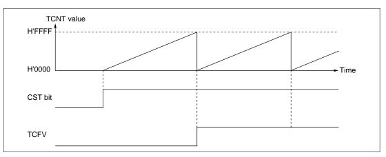
Figure 9.7 illustrates free-running counter operation.
