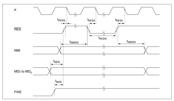
Figure 20.9 Reset Input Timing
