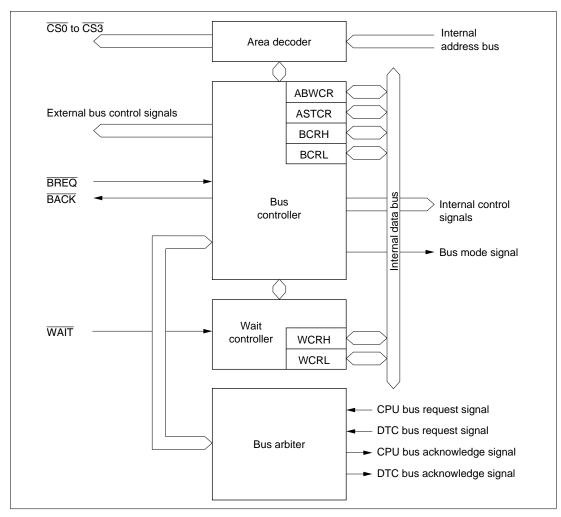
Figure 6.1 Block Diagram of Bus Controller
