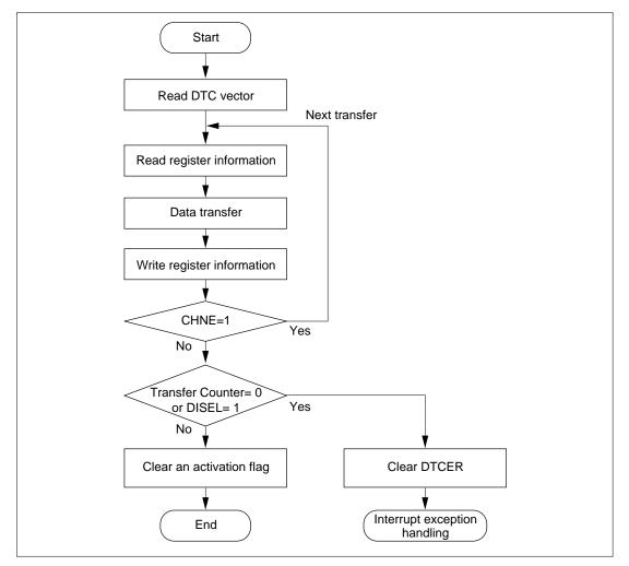
Figure 7.2 Flowchart of DTC Operation
