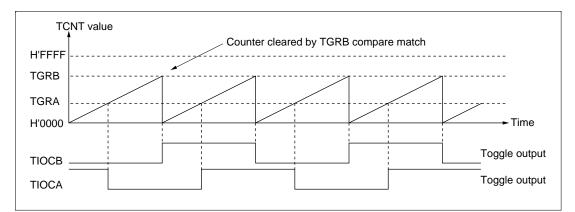
Figure 9.11 Example of Toggle Output Operation
