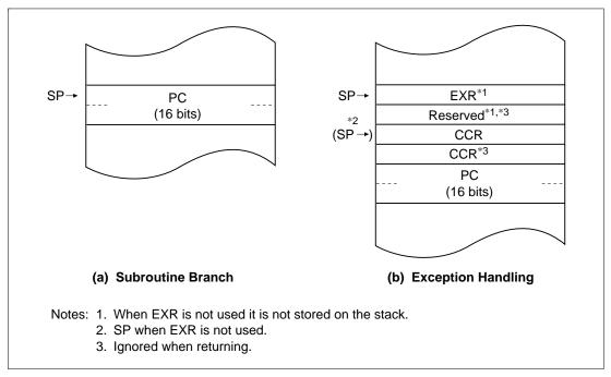
Figure 2.3 Stack Structure in Normal Mode
