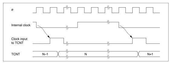
Figure 10.2 Count Timing for Internal Clock Input
