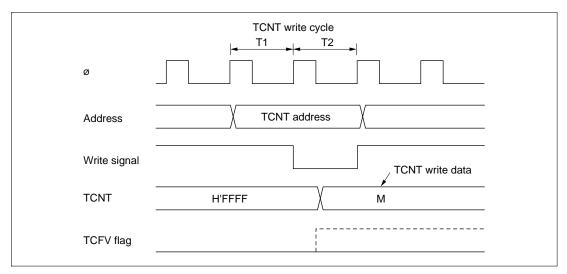
Figure 9.57 Contention between TCNT Write and Overflow
