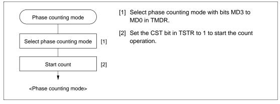
Figure 9.28 Example of Phase Counting Mode Setting Procedure
