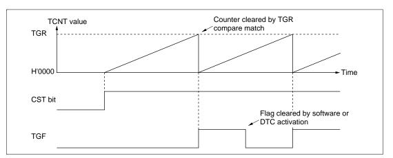
Figure 9.8 illustrates periodic counter operation.
