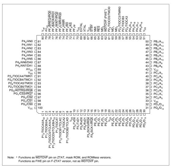
Figure 1.3 Pin Arrangement (FP-100A: Top View)
