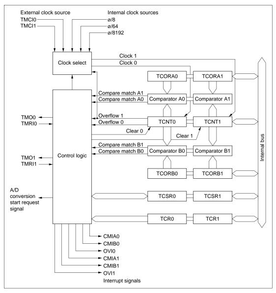
Figure 10.1 Block Diagram of 8-Bit Timer
