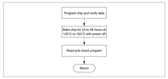
Figure 17.6 Recommended Screening Procedure
