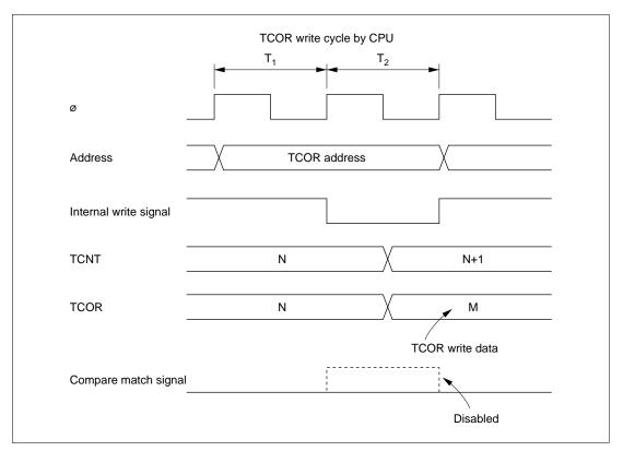
Figure 10.12 Contention between TCOR Write and Compare Match
