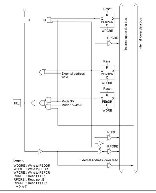
Figure C.9 Port E Block Diagram (Pin PE<sub>n</sub>)
