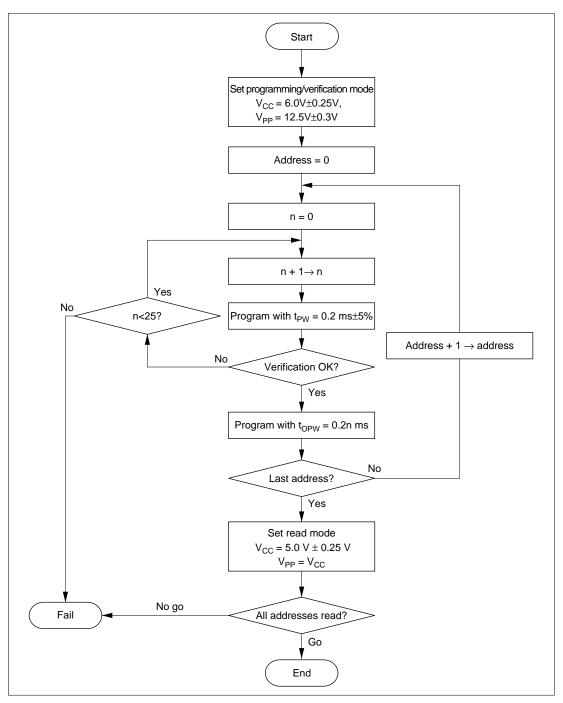
Figure 17.4 High-Speed Programming Flowchart
