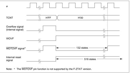
Figure 11.7 Timing of Setting of WOVF
