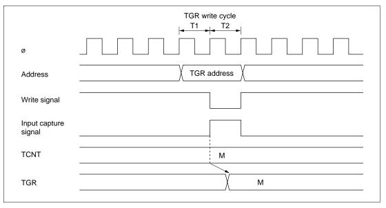
Figure 9.54 Contention between TGR Write and Input Capture
