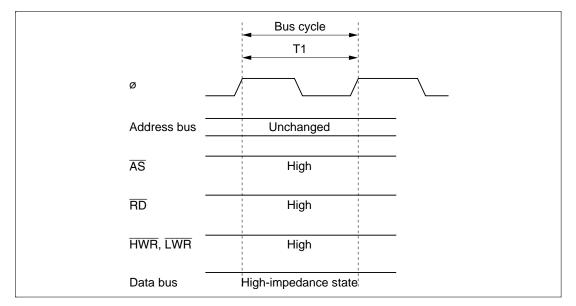
Figure 2.18 Pin States during On-Chip Memory Access
