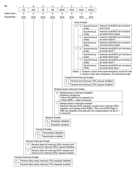
SCR0—Serial Control Register 0
