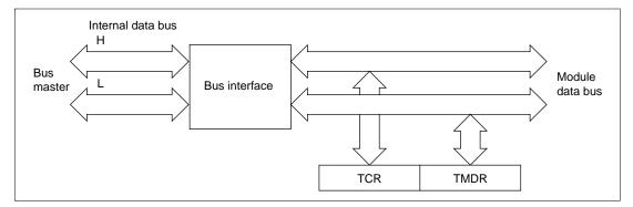
Figure 9.5 8-Bit Register Access Operation [Bus Master \leftrightarrow TCR and TMDR (16 Bits)]
