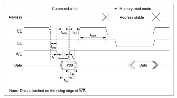
Figure 17.27 Memory Read Mode Transition Timing Waveforms
