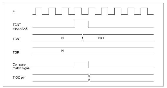
Figure 9.36 Output Compare Output Timing
