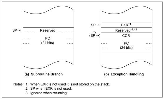
Figure 2.5 Stack Structure in Advanced Mode
