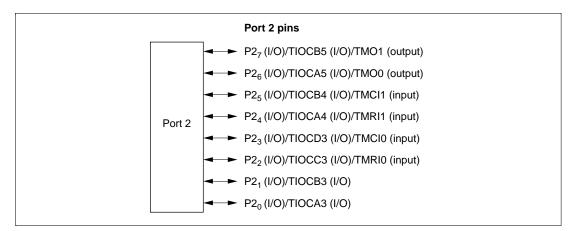
Figure 8.2 Port 2 Pin Functions
