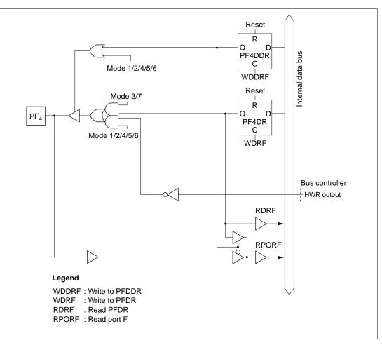
Figure C.10 (e) Port F Block Diagram (Pin PF<sub>4</sub>)
