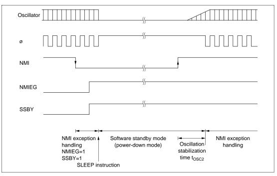
Figure 19.2 Software Standby Mode Application Example
