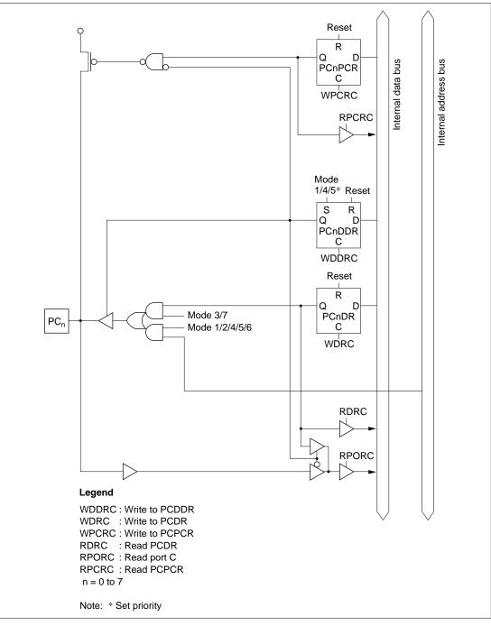
Figure C.7 Port C Block Diagram (Pin PC<sub>n</sub>)
