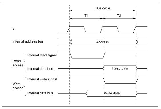
Figure 2.19 On-Chip Supporting Module Access Cycle
