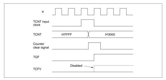
Figure 9.56 Contention between Overflow and Counter Clearing
