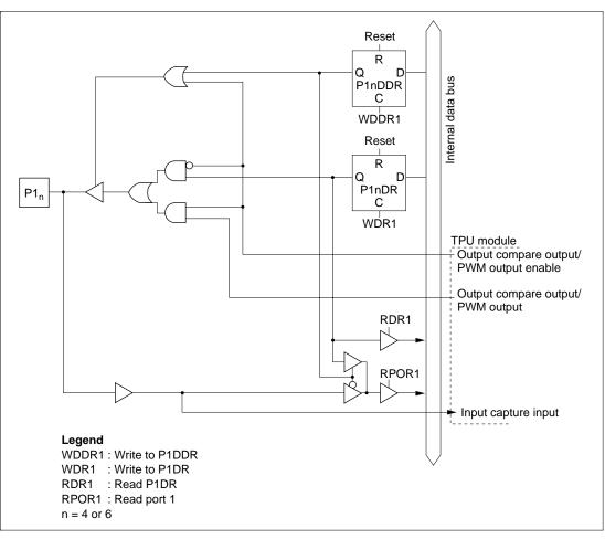
Figure C.1 (c) Port 1 Block Diagram (Pins P1<sub>4</sub> and P1<sub>6</sub>)
