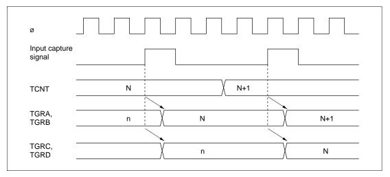
Figure 9.41 Buffer Operation Timing (Input Capture)
