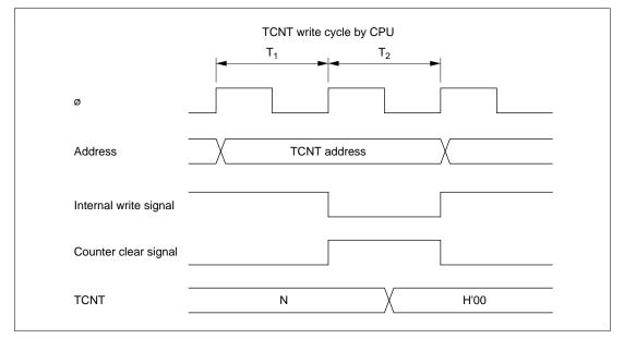
Figure 10.10 Contention between TCNT Write and Clear
