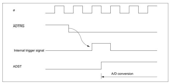
Figure 14.6 External Trigger Input Timing
