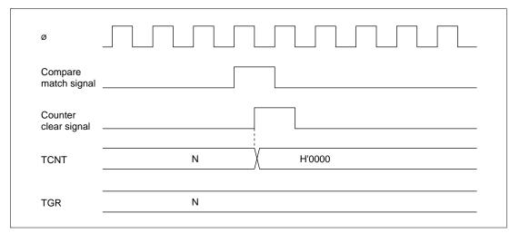
Figure 9.38 Counter Clear Timing (Compare Match)
