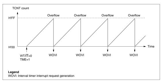
Figure 11.5 Interval Timer Operation
