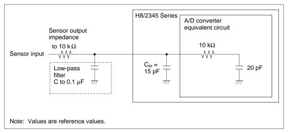
Figure 14.11 Example of Analog Input Circuit
