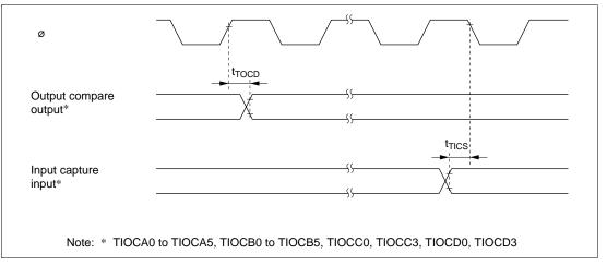
Figure 20.18 TPU Input/Output Timing
