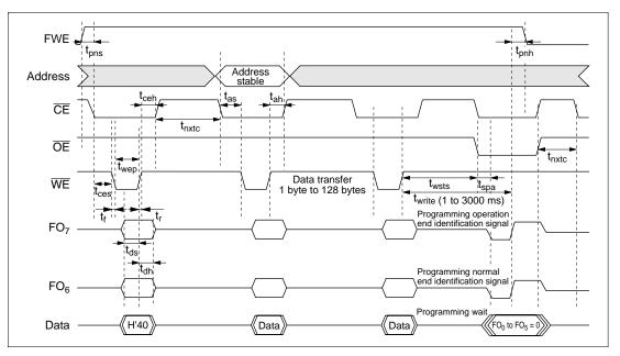
Figure 17.31 Auto-Program Mode Timing Waveforms
