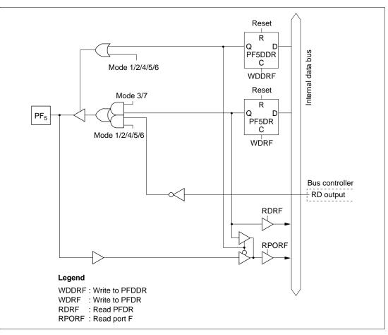
Figure C.10 (f) Port F Block Diagram (Pin PF<sub>5</sub>)
