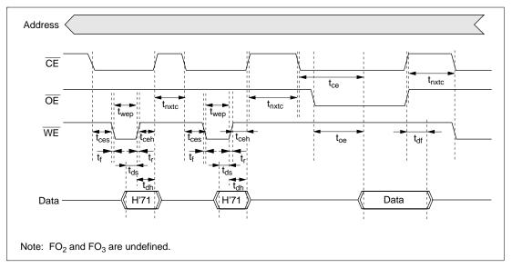
Figure 17.33 Status Read Mode Timing Waveforms
