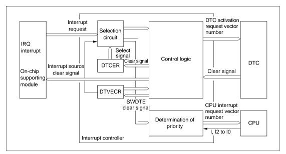
Figure 5.9 Interrupt Control for DTC and DMAC
