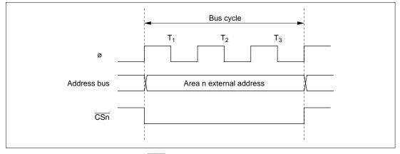
Figure 6.3  $\overline{\text{CSn}}$  Signal Output Timing (n = 0 to 3)
