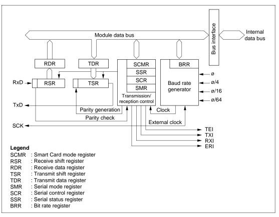
Figure 12.1 Block Diagram of SCI
