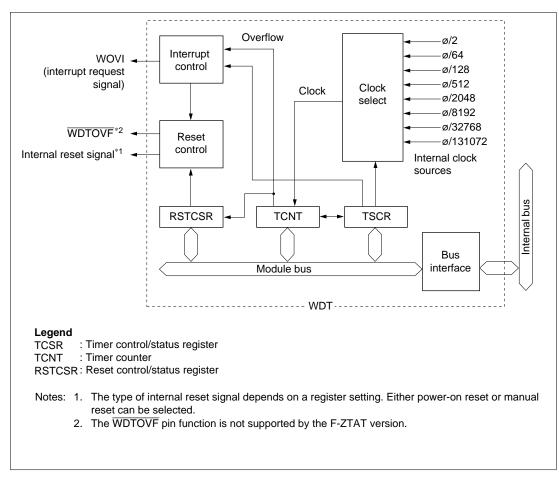
Figure 11.1 Block Diagram of WDT
