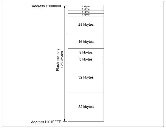
Figure 17.13 Flash Memory Block Configuration
