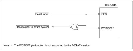
Figure 11.9 Circuit for System Reset by WDTOVF Signal (Example)
