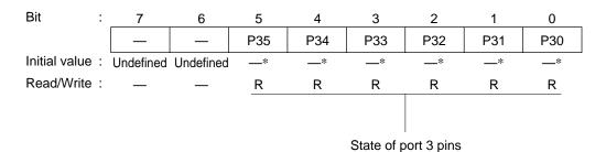
Note: \* Determined by the state of pins  $P3_5$  to  $P3_0$ .
