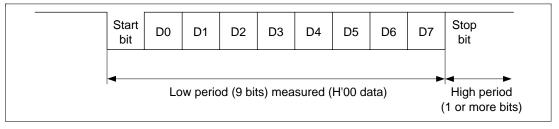
Figure 17.17 Measurement of Low Period of Host Transmission Data
