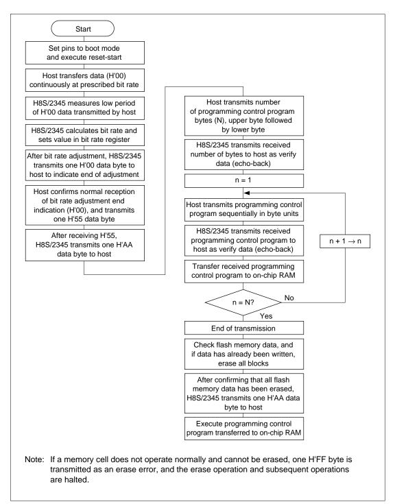
Figure 17.16 Boot Mode Execution Procedure
