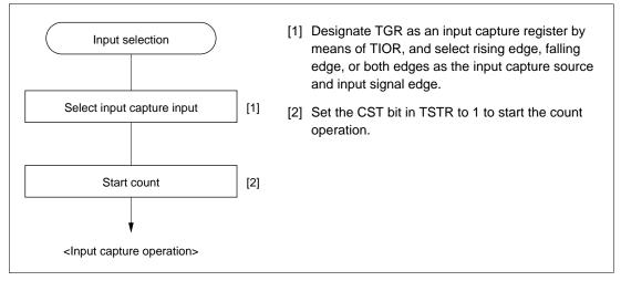
Figure 9.12 Example of Input Capture Operation Setting Procedure
