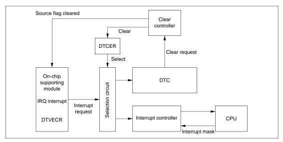
Figure 7.3 Block Diagram of DTC Activation Source Control
