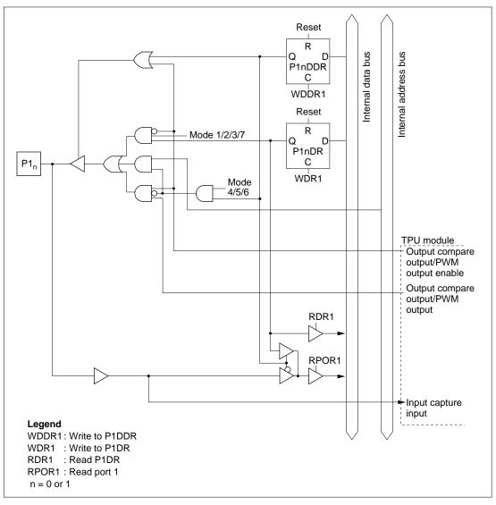
Figure C.1 (a) Port 1 Block Diagram (Pins P1<sub>0</sub> and P1<sub>1</sub>)
