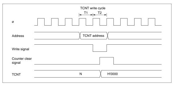
Figure 9.49 Contention between TCNT Write and Clear Operations
