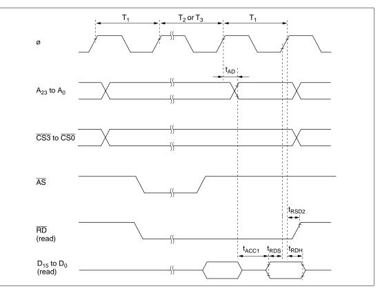
Figure 20.15 Burst ROM Access Timing (One-State Access)
