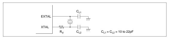
Figure 18.2 Connection of Crystal Resonator (Example)
