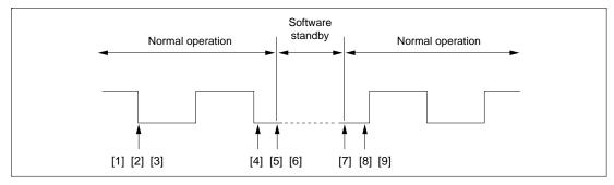
Figure 13.9 Clock Halt and Restart Procedure
