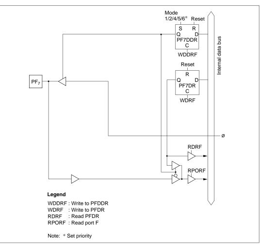
Figure C.10 (h) Port F Block Diagram (Pin PF<sub>7</sub>)
