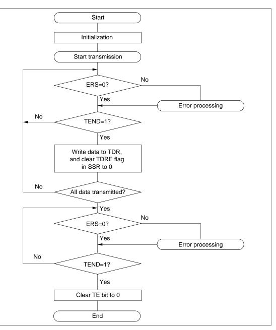
Figure 13.4 Example of Transmission Processing Flow
