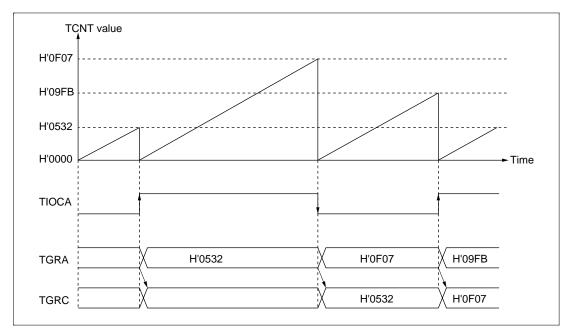
Figure 9.20 Example of Buffer Operation (2)
