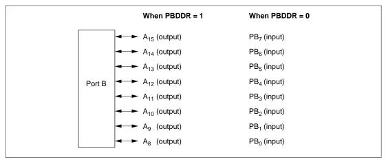
Figure 8.11 Port B Pin Functions (Modes 2 and 6) \*
