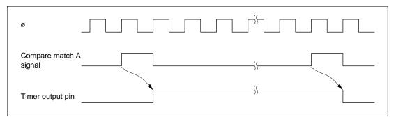
Figure 10.5 Timing of Timer Output
