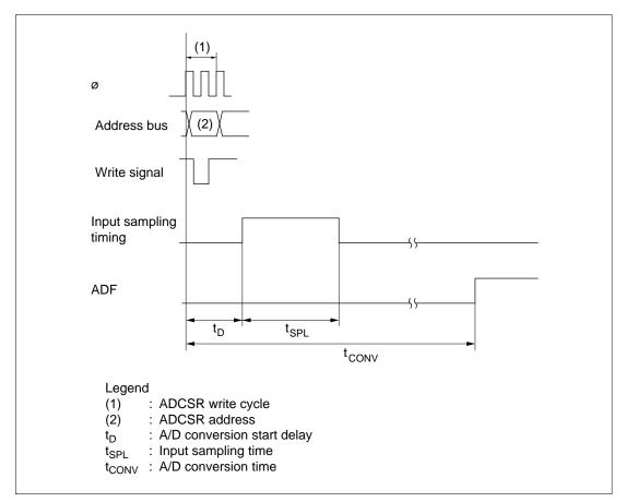
Figure 14.5 A/D Conversion Timing
