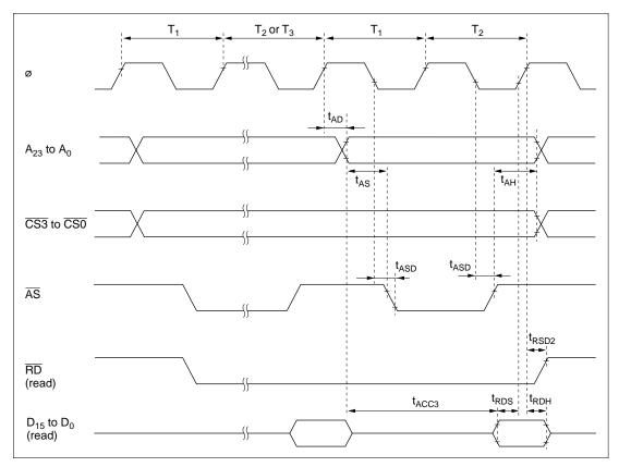
Figure 20.14 Burst ROM Access Timing (Two-State Access)
