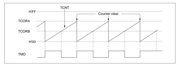
Figure 10.9 Example of Pulse Output
