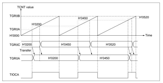
Figure 9.19 Example of Buffer Operation (1)
