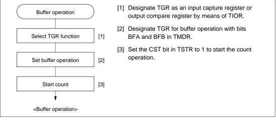
Figure 9.18 Example of Buffer Operation Setting Procedure
