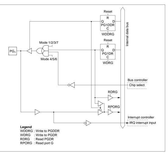
Figure C.11 (b) Port G Block Diagram (Pin PG<sub>1</sub>)
