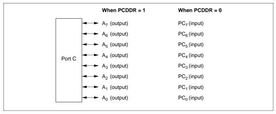
Figure 8.15 Port C Pin Functions (Modes 2 and 6)\*
