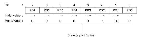
Note: \* Determined by the state of pins PB7 to PB0.
