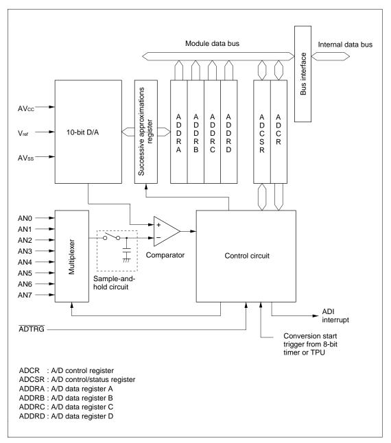
Figure 14.1 Block Diagram of A/D Converter
