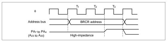
Figure 6.24 BRCR Write Timing
