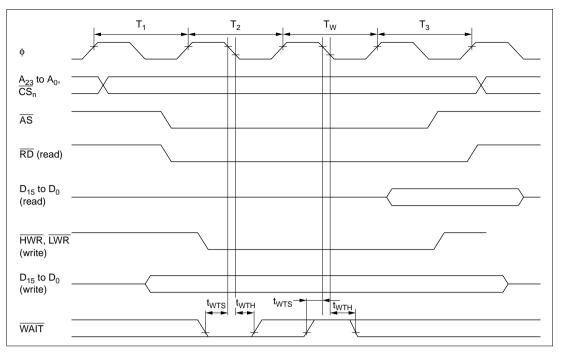
Figure 22.19 Basic Bus Cycle: Three-State Access with One Wait State
