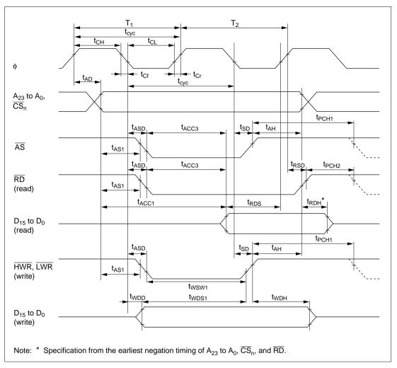
Figure 22.17 Basic Bus Cycle: Two-State Access
