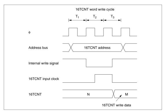
Figure 8.38 Contention between 16TCNT Word Write and Increment
