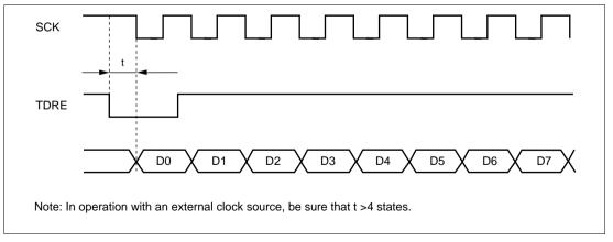
Figure 12.22 Example of Synchronous Transmission
