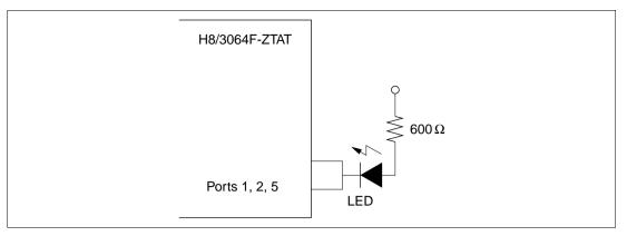
Figure 22.8 Sample LED Circuit
