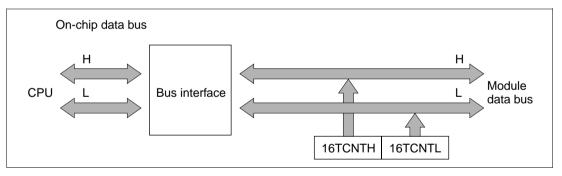
Figure 8.5 Access to Timer Counter (CPU Reads 16TCNT, Word)
