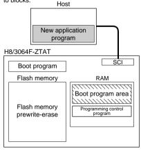
2. Programming control program transfer When boot mode is entered, the boot program in the H8/3064F-ZTAT (originally incorporated in the chip) is started and the programming control program in the host is transferred to RAM via SCI communication. The boot program required for flash memory erasing is automatically transferred to the RAM boot program area.
