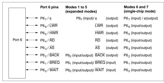
Figure 7.6 Port 6 Pin Configuration
