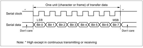
Figure 12.14 Data Format in Synchronous Communication
