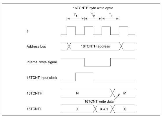
Figure 8.39 Contention between 16TCNT Byte Write and Increment
