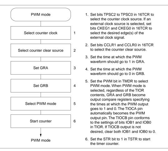
Figure 8.26 Setup Procedure for PWM Mode (Example)
