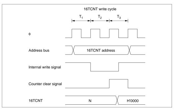
Figure 8.37 Contention between 16TCNT Write and Clear
