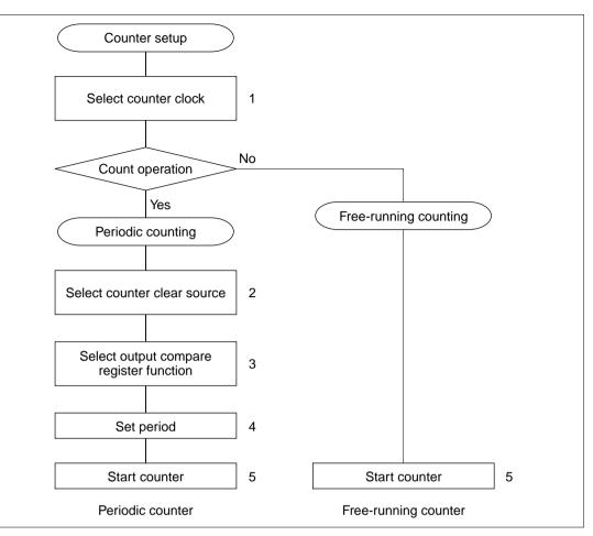
Figure 8.12 Counter Setup Procedure (Example)
