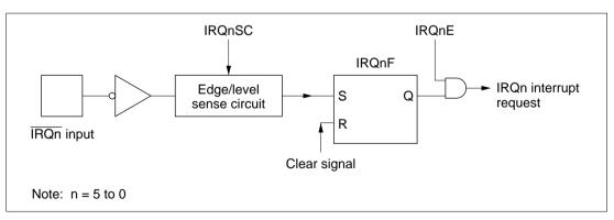
Figure 5.2 shows a block diagram of interrupts IRQ<sub>0</sub> to IRQ<sub>5</sub>.
