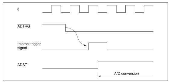
Figure 14.6 External Trigger Input Timing
