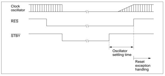
Figure 21.2 Hardware Standby Mode Timing
