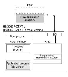
Writing new application program Next, the new application program in the host is written into the erased flash memory blocks. Do not write to unerased blocks.
