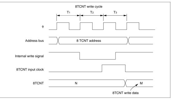
Figure 9.19 Contention between 8TCNT Write and Increment
