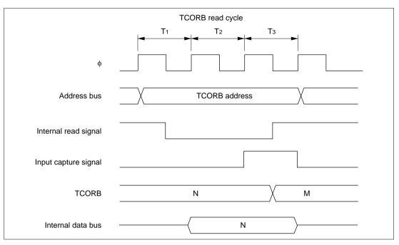
Figure 9.21 Contention between TCOR Read and Input Capture
