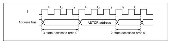
Figure 6.22 ASTCR Write Timing
