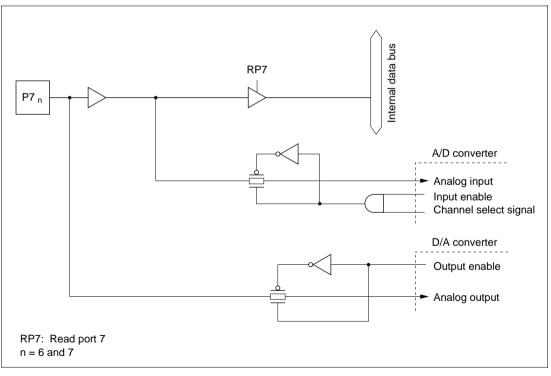
Figure C.7 (b) Port 7 Block Diagram (Pins P7<sub>6</sub> and P7<sub>7</sub>)
