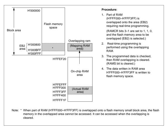
Figure 17.14 Example of RAM Overlap Operation
