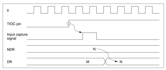
Figure 10.8 TPC Output Triggering by Input Capture (Example)
