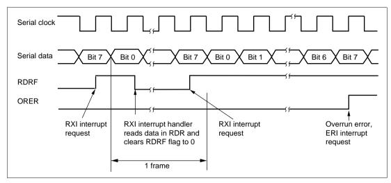
Figure 12.19 Example of SCI Receive Operation
