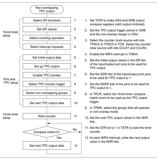
Figure 10.6 Setup Procedure for Non-Overlapping TPC Output (Example)
