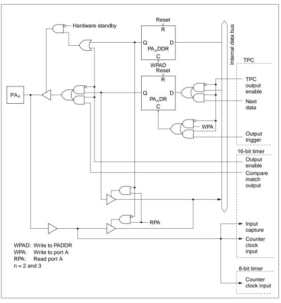
Figure C.10 (b) Port A Block Diagram (Pins PA<sub>2</sub> and PA<sub>3</sub>)
