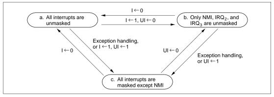
Figure 5.5 Interrupt Masking State Transitions (Example)
