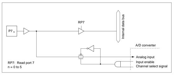
Figure C.7 (a) Port 7 Block Diagram (Pins P7<sub>0</sub> to P7<sub>5</sub>)
