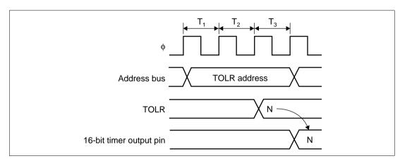
Figure 8.32 Timing for Setting 16-Bit Timer Output Level by Writing to TOLR
