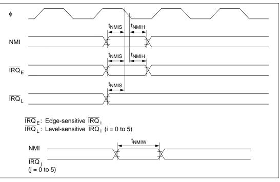
Figure 22.16 Interrupt Input Timing
