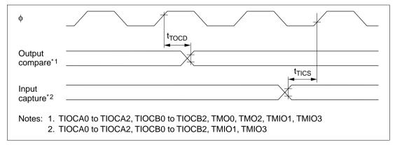
Figure 22.22 Timer Input/Output Timing
