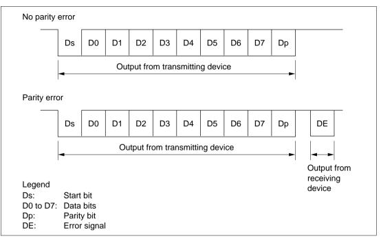
Figure 13.3 Smart Card Interface Data Format
