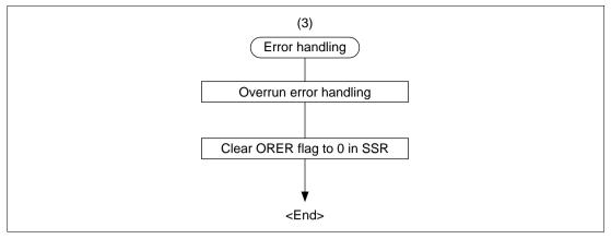
Figure 12.18 Sample Flowchart for Serial Receiving (cont)
