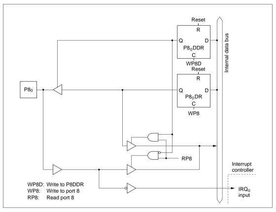
Figure C.8 (a) Port 8 Block Diagram (Pin P8<sub>0</sub>)
