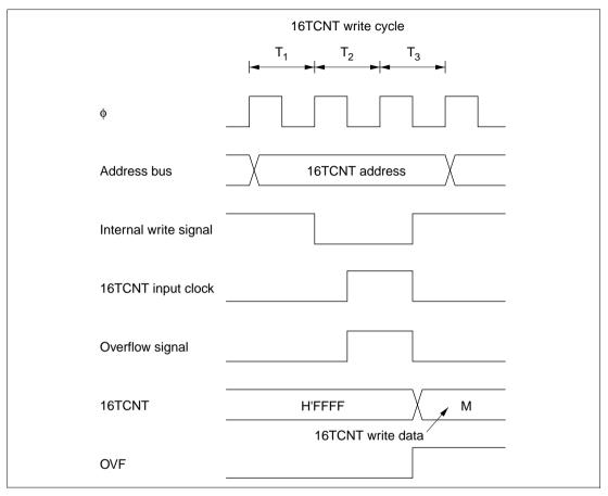
Figure 8.41 Contention between 16TCNT Write and Overflow
