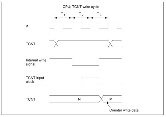
Figure 11.8 Contention between TCNT Write and Count up
