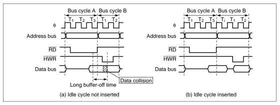
Figure 6.19 Example of Idle Cycle Operation (ICIS0 = 1)
