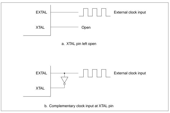
Figure 20.5 External Clock Input (Examples)
