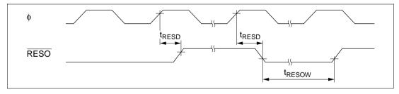
Figure 22.15 Reset Output Timing\*
