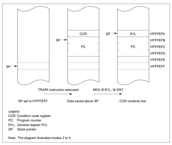
Figure 4.7 Operation when SP Value is Odd
