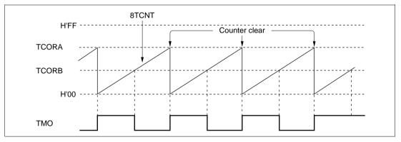
Figure 9.17 Example of Pulse Output
