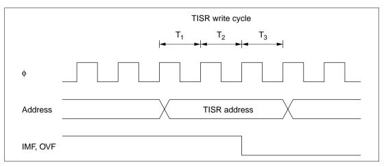
Figure 8.36 Timing of Clearing of Status Flags
