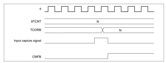
Figure 9.15 CMFB Flag Setting Timing when Input Capture Occurs
