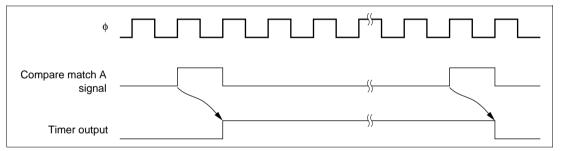
Figure 9.10 Timing of Timer Output
