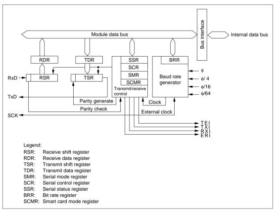
Figure 12.1 SCI Block Diagram
