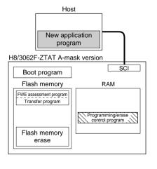
Programming/erase control program transfer When user program mode is entered, user software recognizes this fact, executes the transfer program in the flash memory, and transfers the programming/erase control program to RAM.
