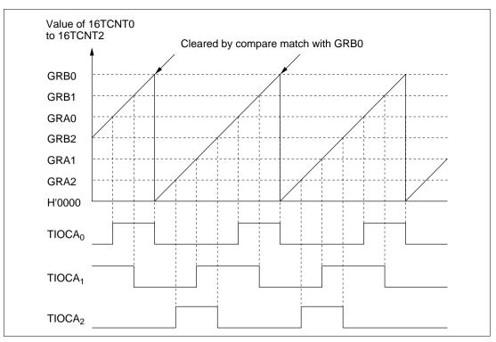
Figure 8.25 Synchronization (Example)
