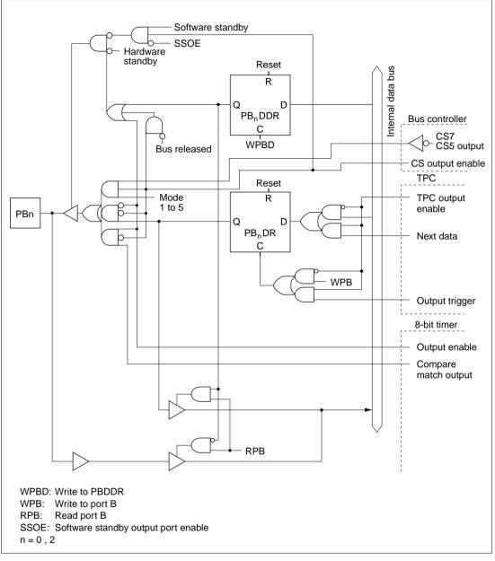
Figure C.11 (a) Port B Block Diagram (Pins PB<sub>0</sub> and PB<sub>2</sub>)
