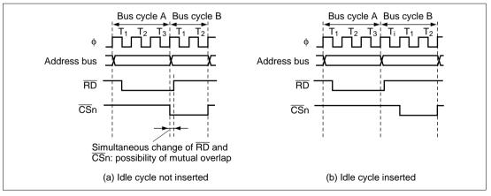
Figure 6.20 Example of Idle Cycle Operation
