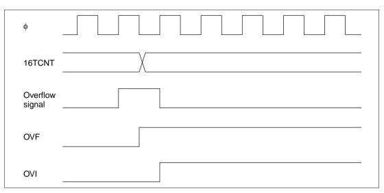
Figure 8.35 Timing of Setting of OVF
