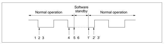
Figure 13.10 Procedure for Stopping and Restarting the Clock
