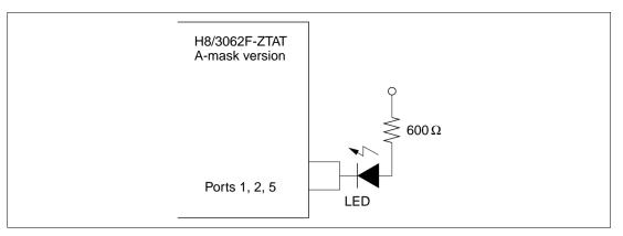
Figure 22.11 Sample LED Circuit
