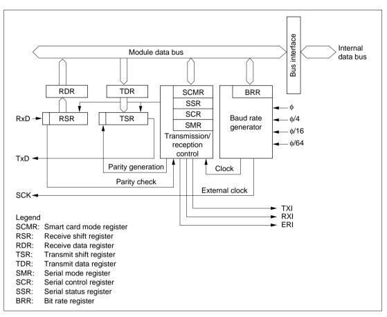
Figure 13.1 Block Diagram of Smart Card Interface
