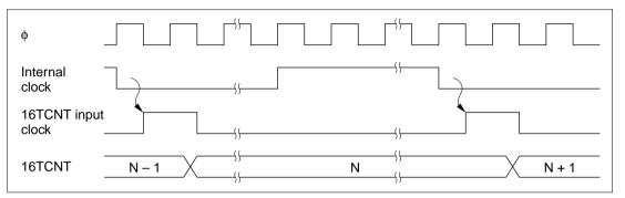
Figure 8.15 Count Timing for Internal Clock Sources
