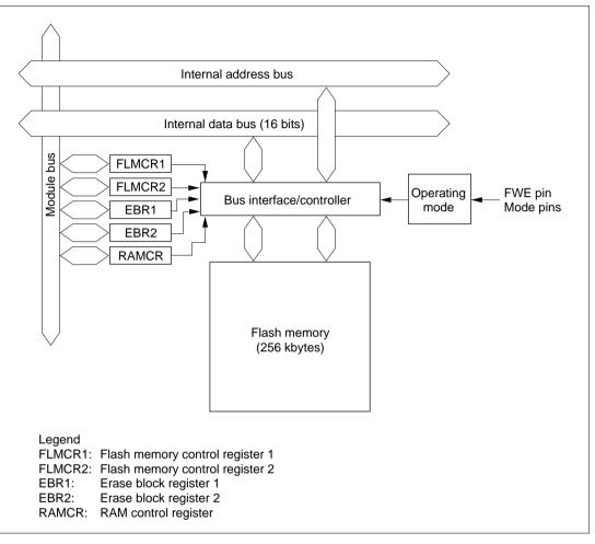
Figure 18.1 Block Diagram of Flash Memory
