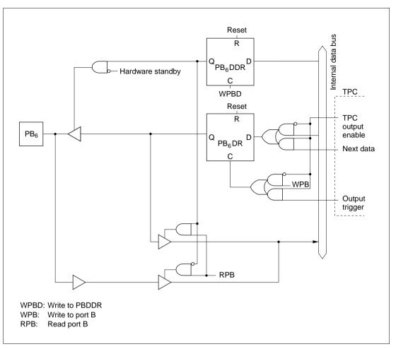
Figure C.11 (e) Port B Block Diagram (Pin PB<sub>6</sub>)
