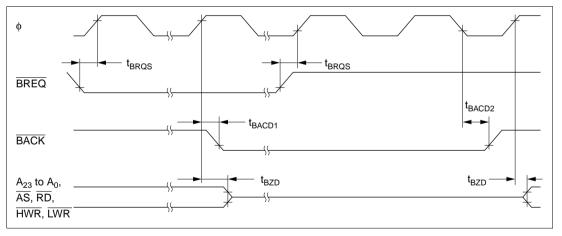
Figure 22.20 Bus-Release Mode Timing
