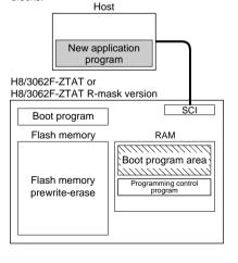
Programming control program transfer When boot mode is entered, the boot program in the H8/3062F-ZTAT or H8/3062F-ZTAT R-mask version (originally incorporated in the chip) is started, an SCI communication check is carried out, and the boot program required for flash memory erasing is automatically transferred to the RAM boot program area.
