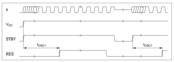
Figure 22.13 Oscillator Settling Timing
