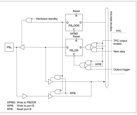
Figure C.11 (c) Port B Block Diagram (Pin PB<sub>4</sub>)
