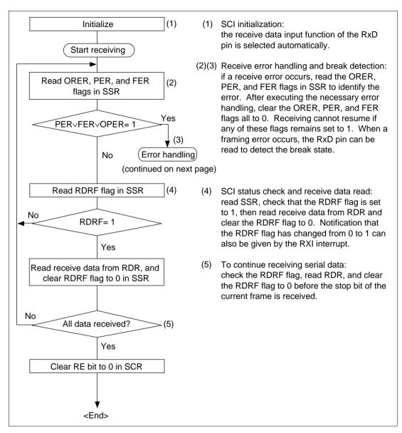
Figure 12.7 Sample Flowchart for Receiving Serial Data
