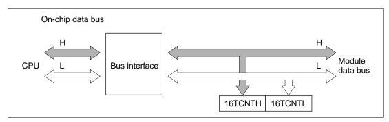
Figure 8.6 Access to Timer Counter H (CPU Writes to 16TCNTH, Upper Byte)
