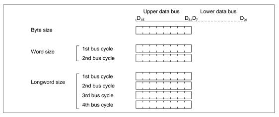
Figure 6.7 Access Sizes and Data Alignment Control (8-Bit Access Area)
