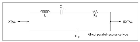
Figure 20.3 Crystal Resonator Equivalent Circuit
