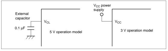
Figure 1.7 Difference between 5 V and 3 V Operation Models
