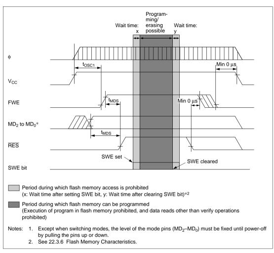
Figure 18.16 Power-On/Off Timing (Boot Mode)
