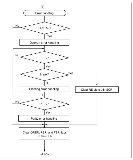
Figure 12.7 Sample Flowchart for Receiving Serial Data (cont)
