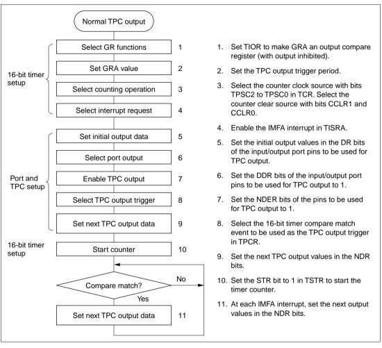
Figure 10.4 Setup Procedure for Normal TPC Output (Example)
