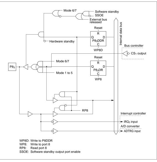
Figure C.8 (c) Port 8 Block Diagram (Pin P83)
