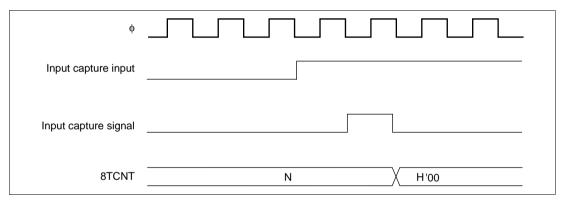
Figure 9.12 Timing of Clear by Input Capture
