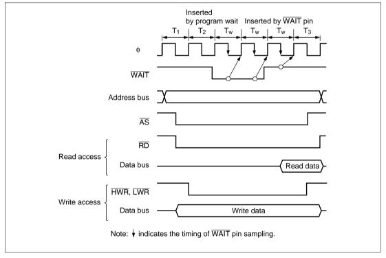
Figure 6.17 Example of Wait State Insertion Timing
