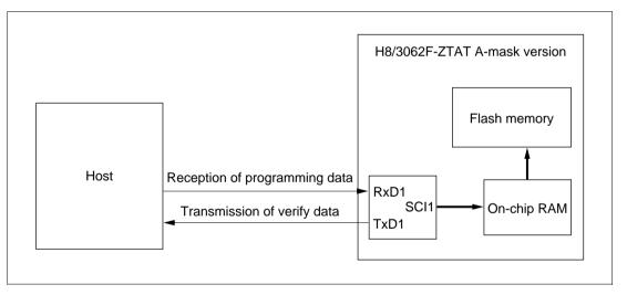
Figure 19.6 System Configuration When Using Boot Mode
