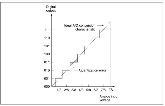
Figure 14.9 A/D Converter Accuracy Definitions (1)
