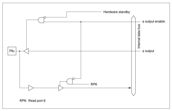
Figure C.6 (e) Port 6 Block Diagram (Pin P67)
