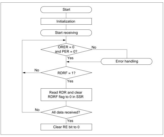
Figure 13.8 Sample Reception Processing Flowchart
