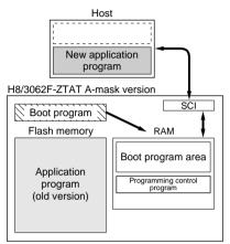
4. Writing new application program An identification check is carried out to see if the programming control program is compatible with the H8/3062F-ZTAT A-mask version. The programming control program transferred from the host to RAM is executed, and the new application program in the host is written into the flash memory.
