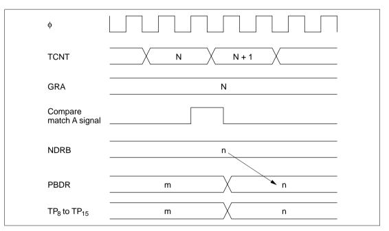
Figure 10.3 Timing of Transfer of Next Data Register Contents and Output (Example)
