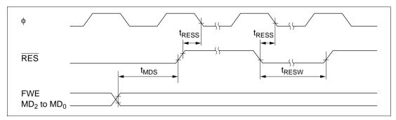
Figure 22.14 Reset Input Timing
