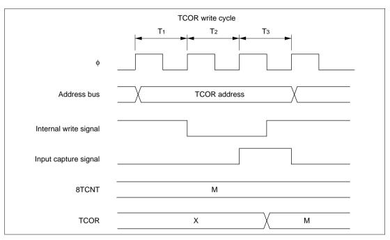
Figure 9.23 Contention between TCOR Write and Input Capture
