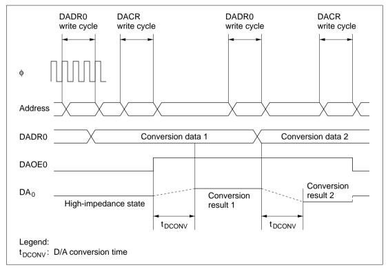
Figure 15.2 Example of D/A Converter Operation
