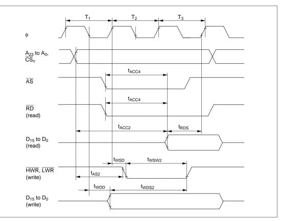
Figure 22.18 Basic Bus Cycle: Three-State Access
