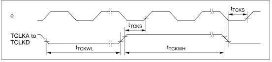
Figure 22.23 Timer External Clock Input Timing
