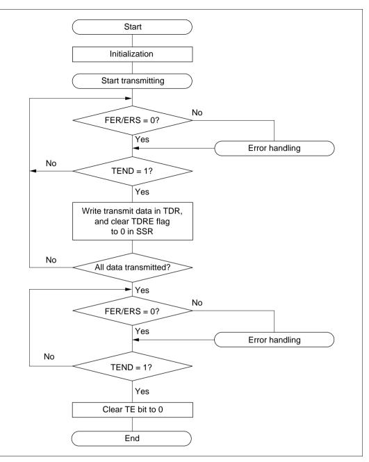
Figure 13.5 Sample Transmission Processing Flowchart
