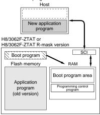
4. Writing new application program The programming control program transferred from the host to RAM by SCI communication is executed, and the new application program in the host is written into the flash memory.
