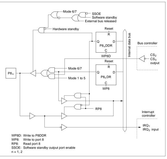
Figure C.8 (b) Port 8 Block Diagram (Pins P8<sub>1</sub> and P8<sub>2</sub>)
