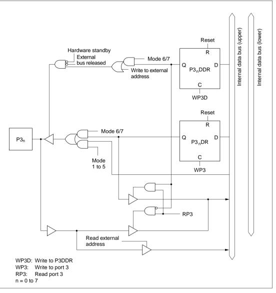
Figure C.3 Port 3 Block Diagram
