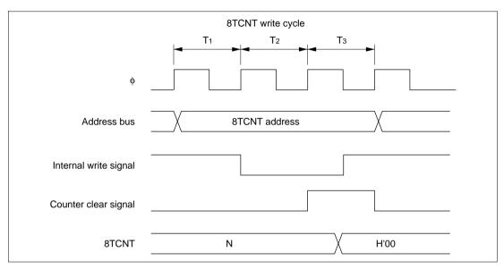
Figure 9.18 Contention between 8TCNT Write and Clear
