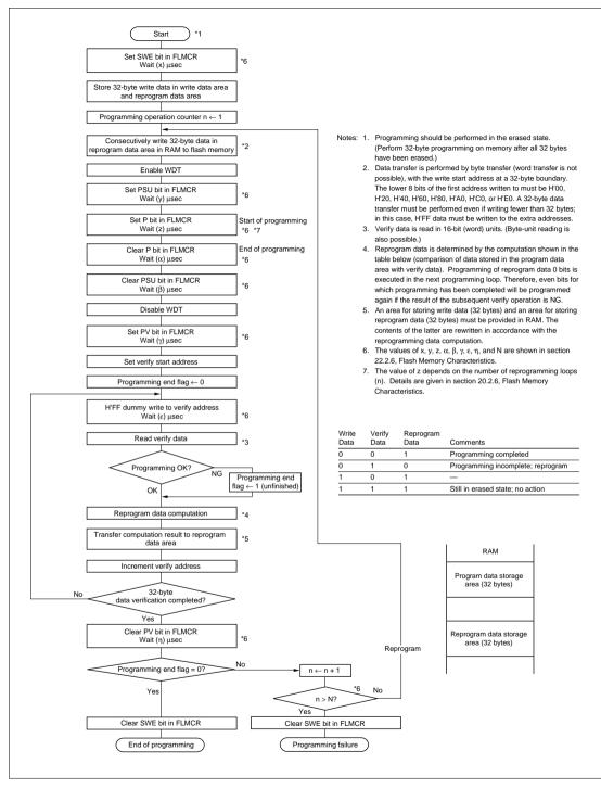
Figure 17.11 Program/Program-Verify Flowchart (32-byte Programming)
