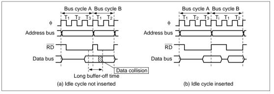
Figure 6.18 Example of Idle Cycle Operation (ICIS1 = 1)
