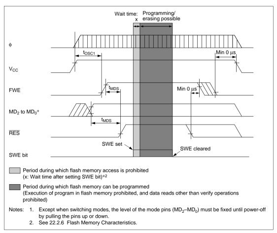
Figure 17.16 Power-On/Off Timing (Boot Mode)
