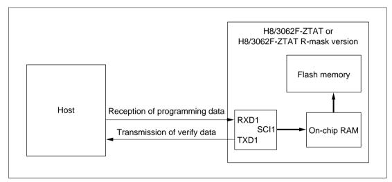
Figure 17.5 System Configuration When Using Boot Mode
