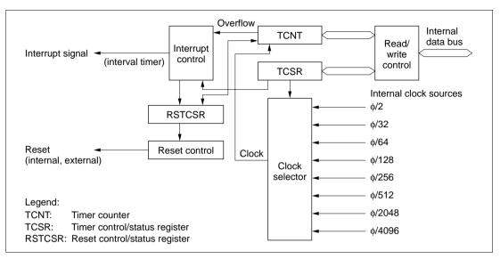
Figure 11.1 WDT Block Diagram
