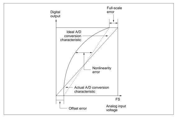
Figure 14.10 A/D Converter Accuracy Definitions (2)
