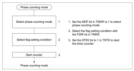
Figure 8.29 Setup Procedure for Phase Counting Mode (Example)
