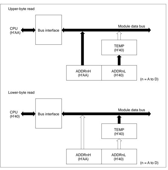
Figure 14.2 A/D Data Register Access Operation (Reading H'AA40)
