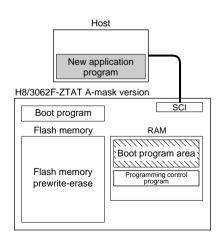
Programming control program transfer When boot mode is entered, the boot program in the H8/3062F-ZTAT A-mask version (originally incorporated in the chip) is started and the programming control program in the host is transferred to RAM via SCI communication. The boot program required for flash memory erasing is automatically transferred to the RAM boot program area.
