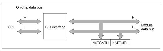
Figure 8.4 16TCNT Access Operation [CPU  $\rightarrow$  16TCNT (Word)]
