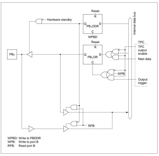
Figure C.11 (f) Port B Block Diagram (Pin PB<sub>7</sub>)
