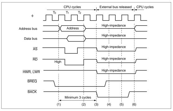
Figure 6.21 Example of External Bus Master Operation
