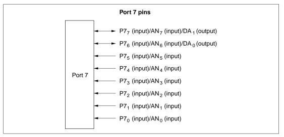
Figure 7.7 Port 7 Pin Configuration
