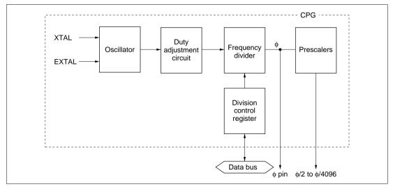
Figure 20.1 Block Diagram of Clock Pulse Generator
