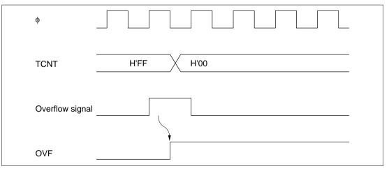
Figure 11.6 Timing of Setting of OVF
