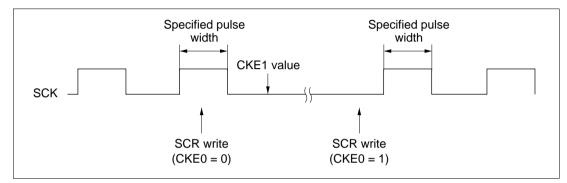
Figure 13.9 Timing for Fixing Cock Output
