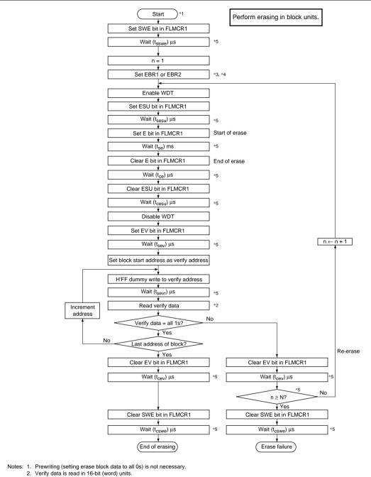
3. Make only a single-bit specification in the erase block registers (EBR1 and EBR2). Two or more bits must not be set simultaneously.
