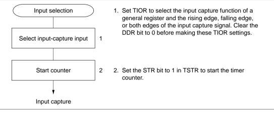
Figure 8.21 Setup Procedure for Input Capture (Example)
