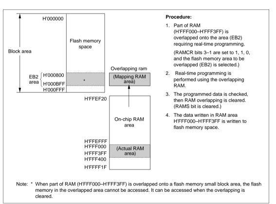
Figure 19.14 Example of RAM Overlap Operation
