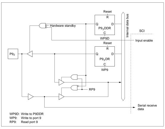
Figure C.9 (c) Port 9 Block Diagram (Pin P9<sub>2</sub>)
