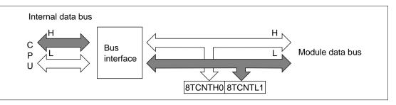
Figure 9.5 8TCNT1 Access Operation (CPU Writes to 8TCNT1, Lower Byte)
