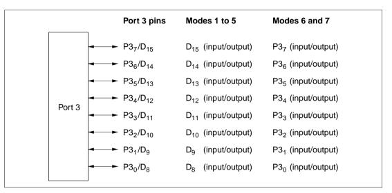
Figure 7.3 Port 3 Pin Configuration
