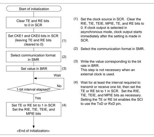
Figure 12.4 Sample Flowchart for SCI Initialization
