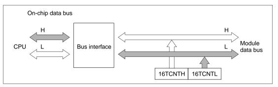
Figure 8.9 Access to Timer Counter L (CPU Reads 16TCNTL, Lower Byte)
