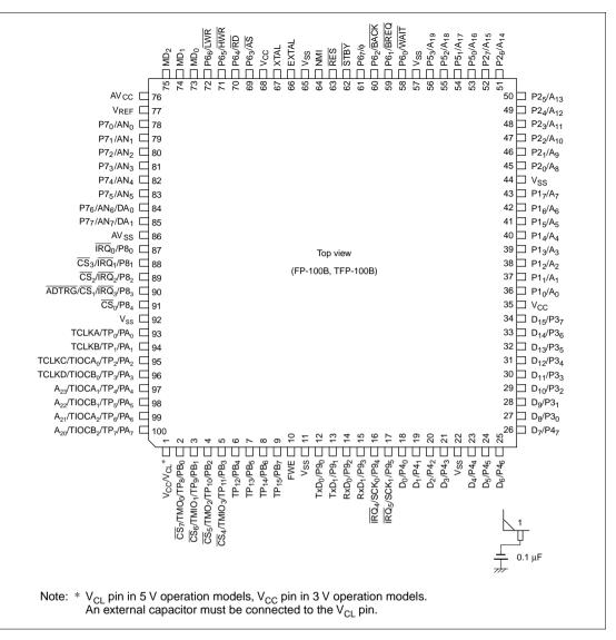
Figure 1.4 Pin Arrangement of H8/3064F-ZTAT and H8/3062F-ZTAT A-Mask Version (FP-100B or TFP-100B Package, Top View)
