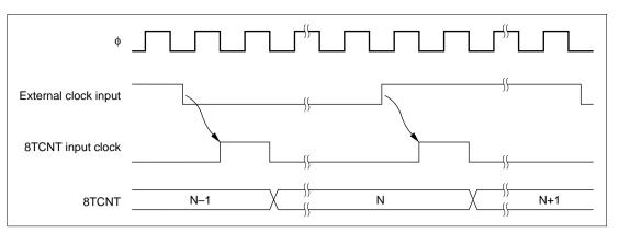
Figure 9.9 Count Timing for External Clock Input (Both-Edge Detection)
