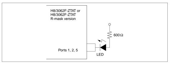
Figure 22.5 Sample LED Circuit
