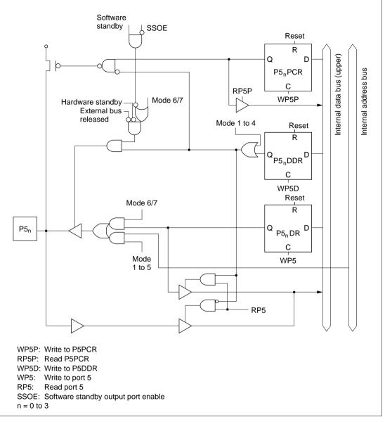
Figure C.5 Port 5 Block Diagram
