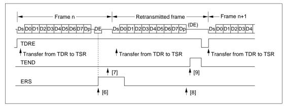
Figure 13.13 Retransmission in SCI Transmit Mode
