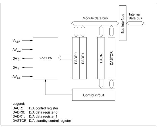
Figure 15.1 D/A Converter Block Diagram
