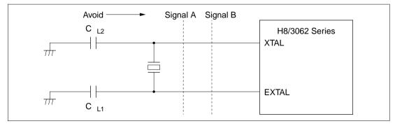
Figure 20.4 Oscillator Circuit Block Board Design Precautions
