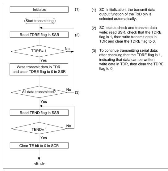
Figure 12.16 Sample Flowchart for Serial Transmitting
