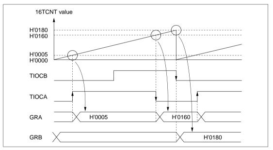
Figure 8.22 Input Capture (Example)
