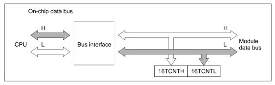
Figure 8.7 Access to Timer Counter L (CPU Writes to 16TCNTL, Lower Byte)
