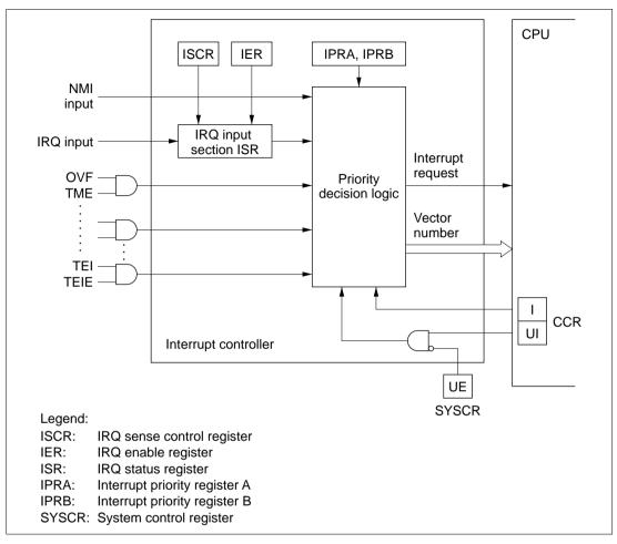
Figure 5.1 Interrupt Controller Block Diagram
