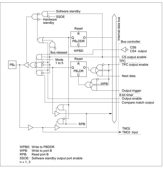
Figure C.11 (b) Port B Block Diagram (Pins PB<sub>1</sub> and PB<sub>3</sub>)
