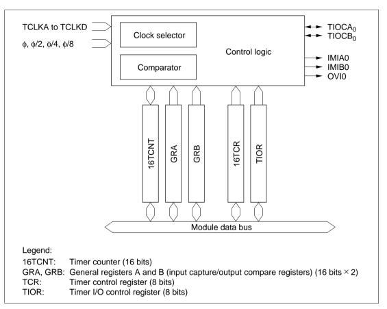
Figure 8.2 Block Diagram of Channels 0 and 1
