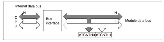
Figure 9.4 8TCNT0 Access Operation (CPU Writes to 8TCNT0, Upper Byte)
