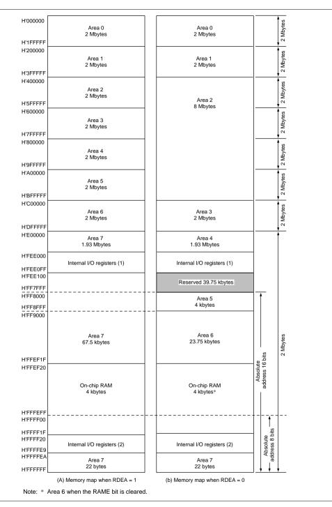
Figure 6.3 Memory Map in 16-Mbyte Mode (H8/3062F-ZTAT, H8/3062F-ZTAT A-Mask Version, H8/3062 Mask ROM Version, H8/3061 Mask ROM Version) (1)
