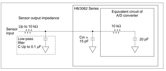
Figure 14.11 Analog Input Circuit (Example)
