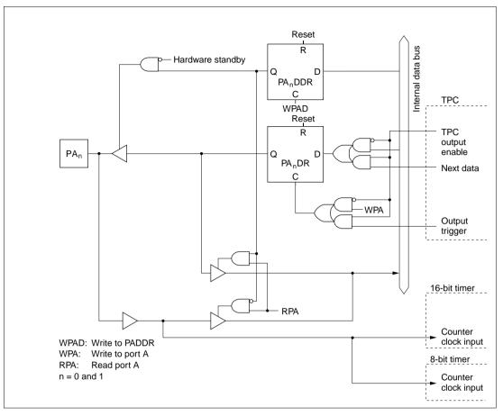
Figure C.10 (a) Port A Block Diagram (Pins PA<sub>0</sub> and PA<sub>1</sub>)
