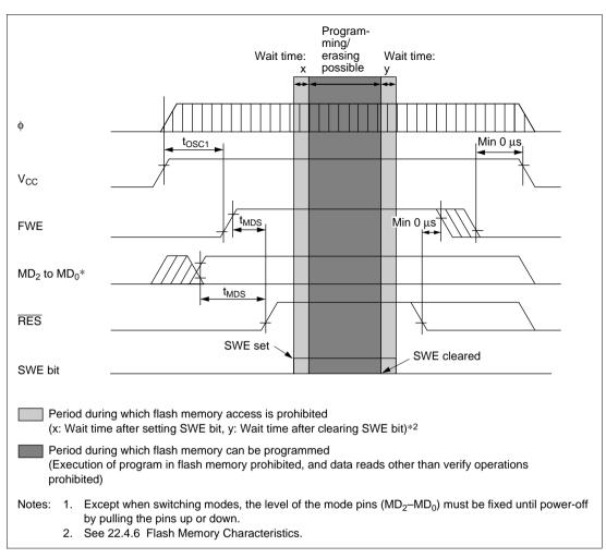
Figure 19.16 Power-On/Off Timing (Boot Mode)
