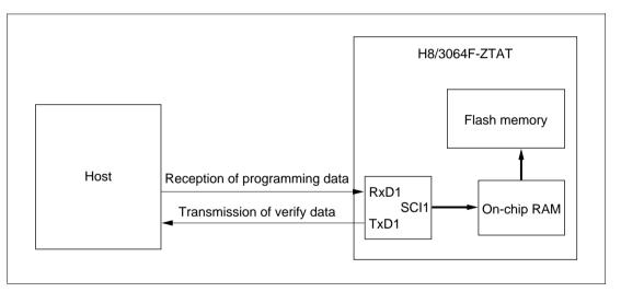
Figure 18.5 System Configuration When Using Boot Mode
