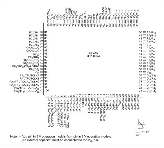
Figure 1.5 Pin Arrangement of H8/3064F-ZTAT and H8/3062F-ZTAT A-Mask Version (FP-100A Package, Top View)
