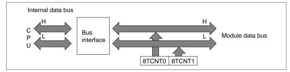
Figure 9.3 8TCNT Access Operation (CPU Reads 8TCNT, Word)
