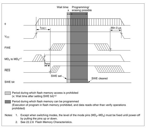
Figure 17.17 Power-On/Off Timing (User Program Mode)
