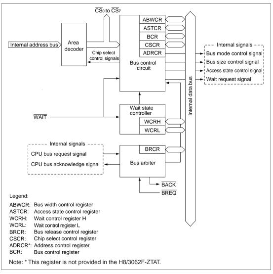
Figure 6.1 Block Diagram of Bus Controller
