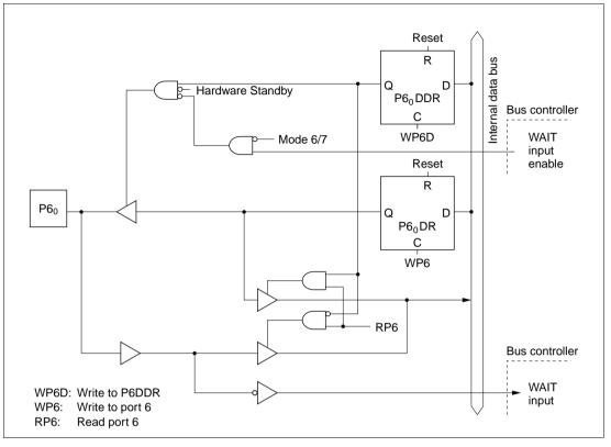
Figure C.6 (a) Port 6 Block Diagram (Pin P6<sub>0</sub>)
