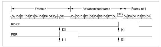
Figure 13.12 Retransmission in SCI Receive Mode
