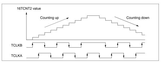
Figure 8.30 Operation in Phase Counting Mode (Example)
