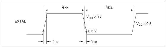
Figure 20.6 External Clock Input Timing
