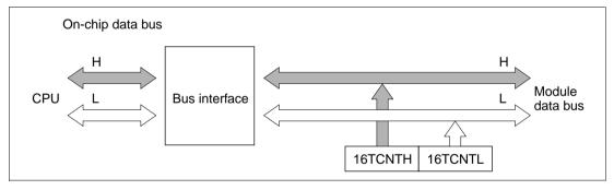
Figure 8.8 Access to Timer Counter H (CPU Reads 16TCNTH, Upper Byte)
