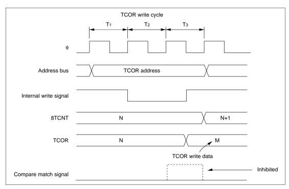
Figure 9.20 Contention between TCOR Write and Compare Match
