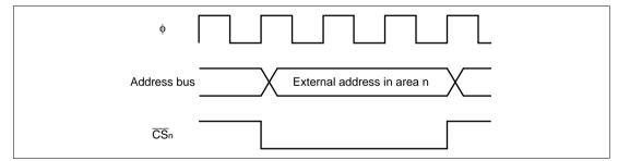
**Figure 6.4**  $\overline{\text{CS}}$ n Signal Output Timing (n = 0 to 7)
