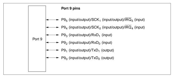
Figure 7.9 Port 9 Pin Configuration
