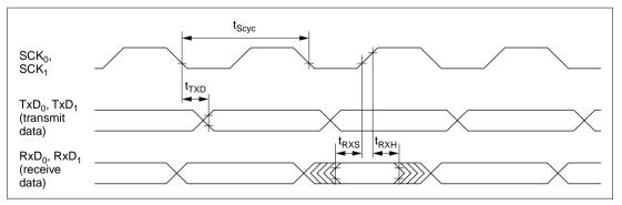
Figure 22.25 SCI Input/Output Timing in Synchronous Mode
