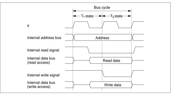
Figure 2.15 On-Chip Memory Access Cycle
