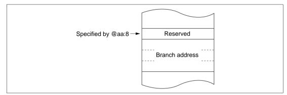
Figure 2.10 Memory-Indirect Branch Address Specification
