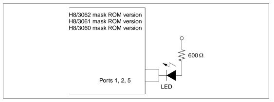
Figure 22.2 Sample LED Circuit
