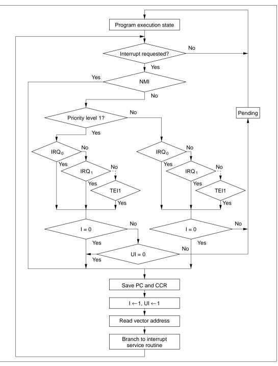
Figure 5.6 Process Up to Interrupt Acceptance when UE = 0
