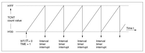
Figure 11.5 Interval Timer Operation
