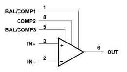
Pin numbers shown are for the D, JG, P, and PS packages.
