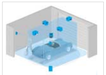
Fig. 1-9: Checking overhang in automated multi-storey car parks
