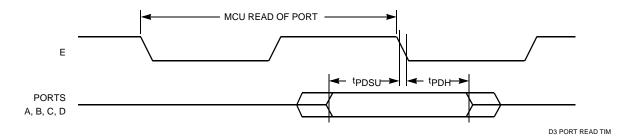
Figure A-7 Port Read Timing Diagram
