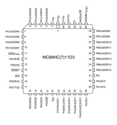
Figure 2-1 Pin Assignments for 44-Pin PLCC
