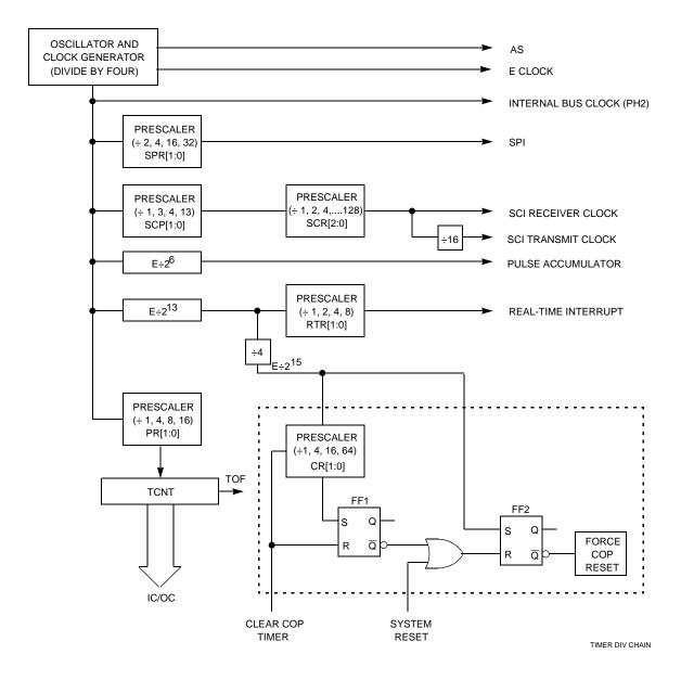
Figure 9-1 Timer Clock Divider Chains
