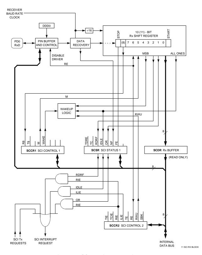
Figure 7-2 SCI Receiver Block Diagram
