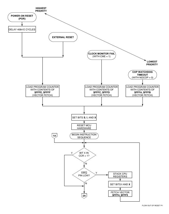
Figure 5-1 Processing Flow out of Reset (1 of 2)
