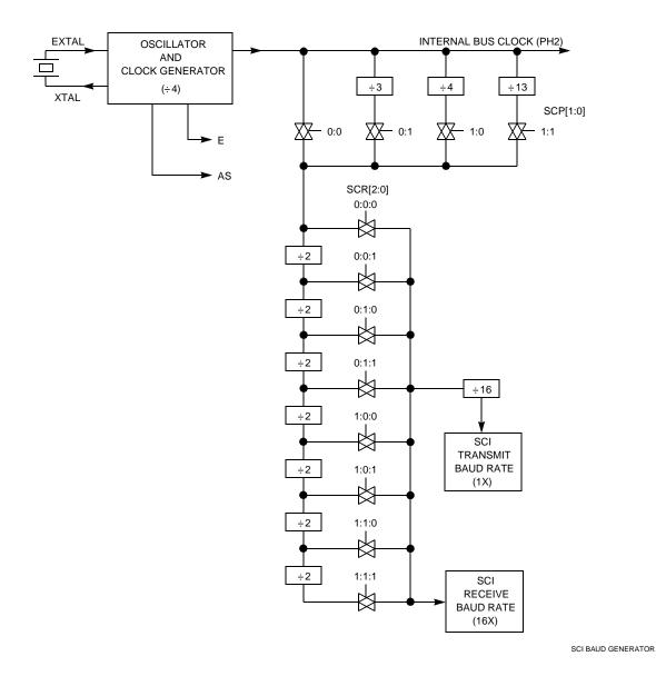
Figure 7-3 SCI Baud Rate Diagram
