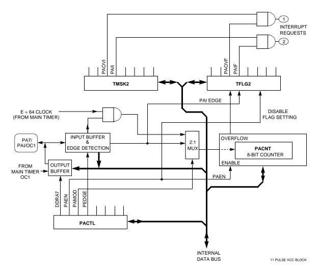
Figure 9-3 Pulse Accumulator
