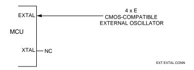
Figure 2-5 External Oscillator Connections
