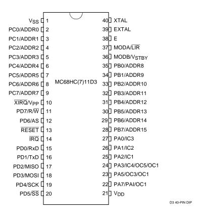
Figure 2-2 Pin Assignments for 40-Pin DIP
