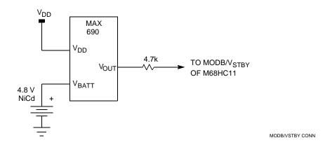
Figure 4-3 RAM Standby MODB/V<sub>STBY</sub> Connections
