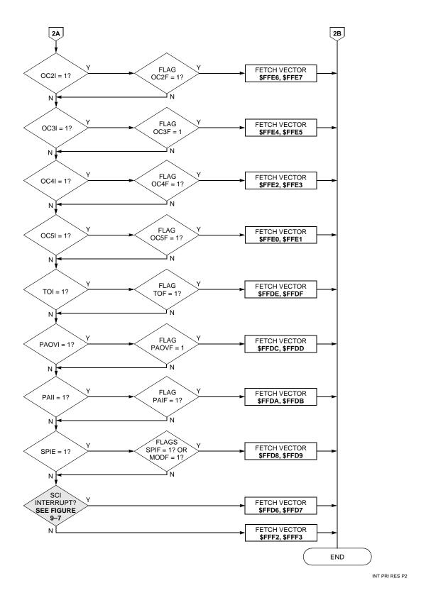
Figure 5-2 Interrupt Priority Resolution (2 of 2)
