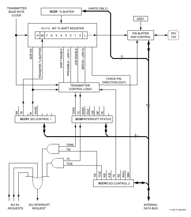
Figure 7-1 SCI Transmitter Block Diagram
