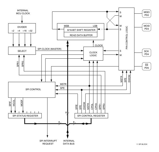
Figure 8-1 SPI Block Diagram
