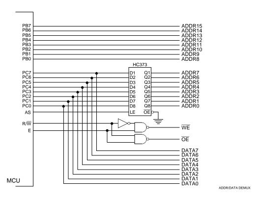
Figure 4-1 Address/Data Demultiplexing
