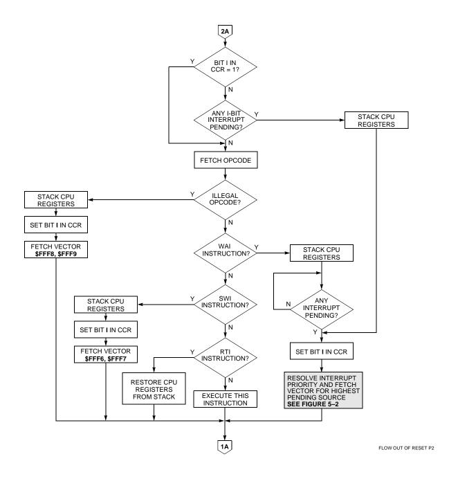
Figure 5-1 Processing Flow out of Reset (2 of 2)
