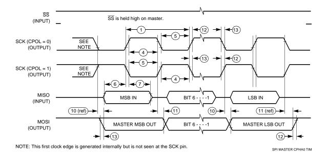
Figure A-9 SPI Master Timing (CPHA = 0)
