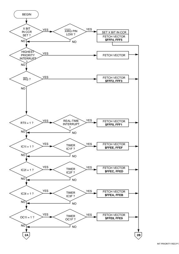
Figure 5-2 Interrupt Priority Resolution (1 of 2)
