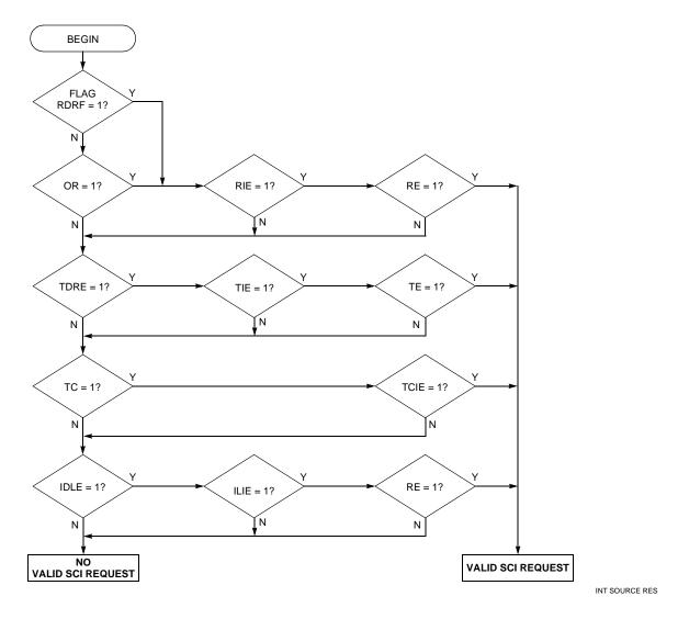
Figure 5-3 Interrupt Source Resolution within SCI
