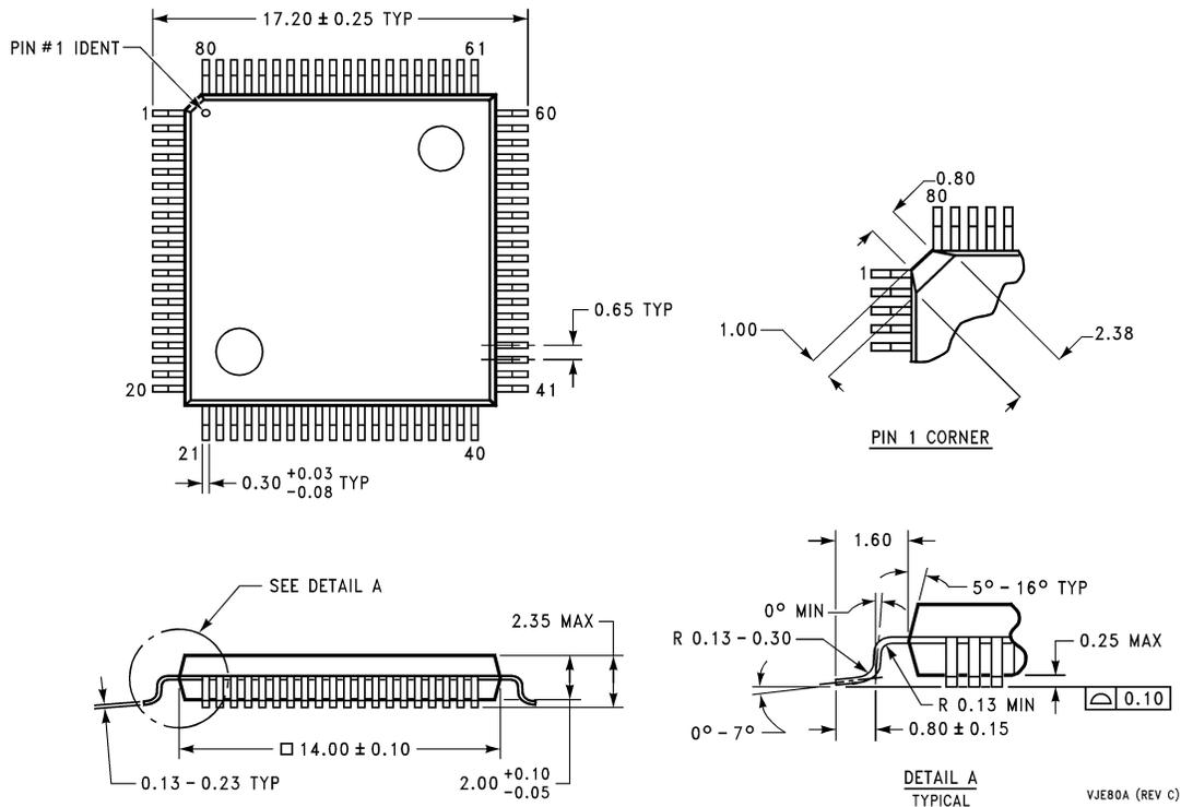
**80 Lead Molded Plastic Quad Flat Package**
