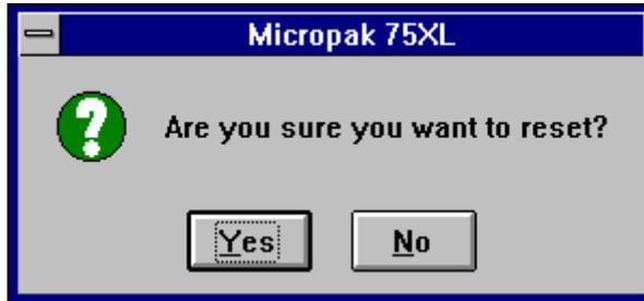
A reset generated in this way will set the processor back to a clock value of '0' and all the normal processor actions expected at reset will occur.
