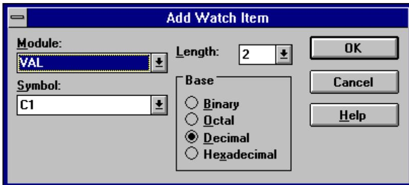
Here items can be selected by choosing module names and symbol names from selection lists. The length of the item can also be specified as can the base to be used for the display of the contents.
