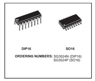
Each device includes an on-ship reference, error amplifier, programmable oscillator, pulse-steering flip flop, two uncommitted output transistors, a high-gain comparator, and current-limiting and shut-down circuitry.
