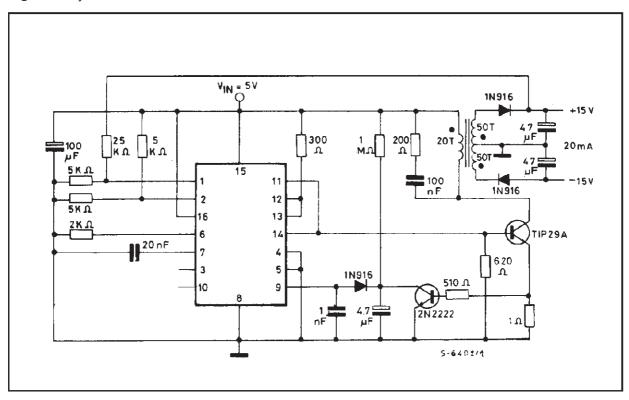
Figure 8: PUSH-PULL Transformer-coupled circuit.
