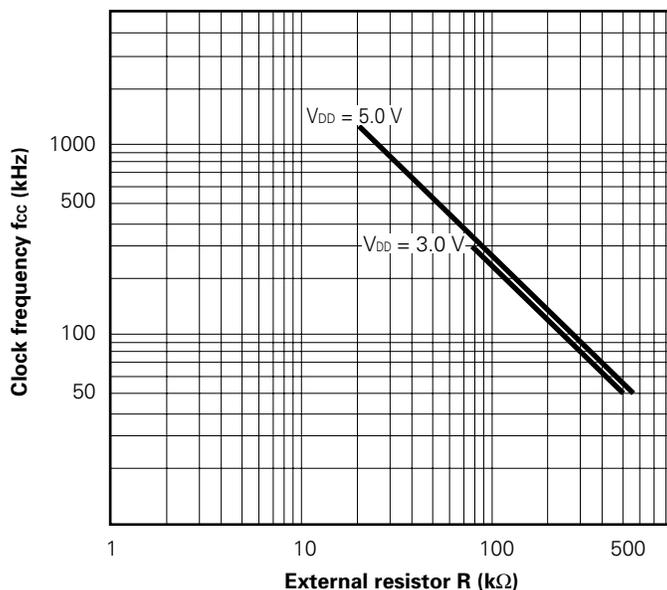
Typical Characteristics:  $f_{cc}$  vs.  $V_{DD}$  ( $T_A = -40$  to  $+85$  °C)
