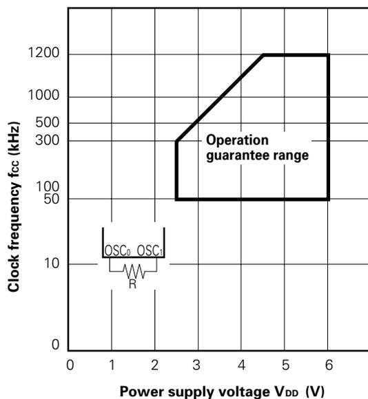
R vs. V<sub>DD</sub> for Operation Guarantee Range (T<sub>A</sub> = -40 to +85 °C)
