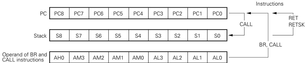
In Fig. 2-1, AH<sub>n</sub>, AM<sub>n</sub>, and AL<sub>n</sub> (n = 0 to 3) indicate bit positions in a 16-bit instruction as follows:
