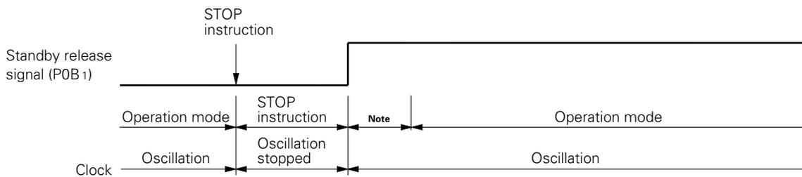
**Note** The HALT mode remains effective in this period, waiting for the generation of clock pulses to settle. At least eight clock pulses on the OSC<sub>1</sub> pin cause operation to start.
