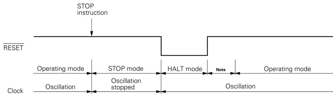
As soon as the  $\overline{\text{RESET}}$  input makes a transition from high to low in the STOP mode, the system clock starts generating clock pulses.
