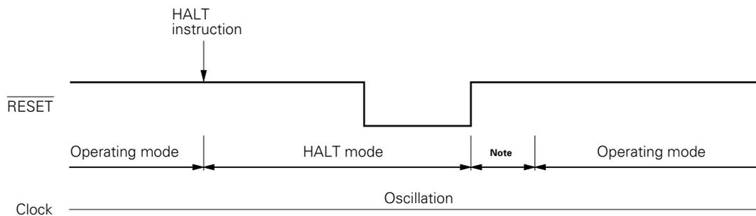
When the RESET signal is applied to release the HALT mode, the  $\overline{\text{RESET}}$  input makes a transition from low to high, then an operating mode is entered.
