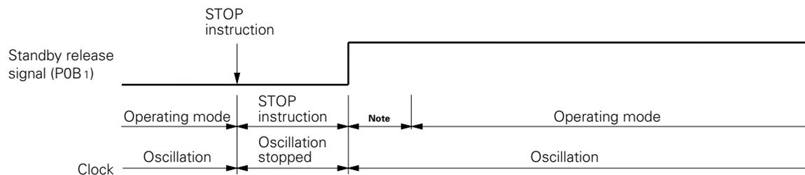
**Note** The HALT mode remains effective in this period, waiting for the generation of clock pulses to settle. An operation starts after eight clock pulses on the OSC<sub>1</sub> pin are counted.
