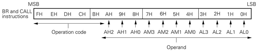
When the assembler (AS17K) is not used and a BR or CALL instruction is used, AH<sub>2</sub> and AH<sub>1</sub> must be set to 0.
