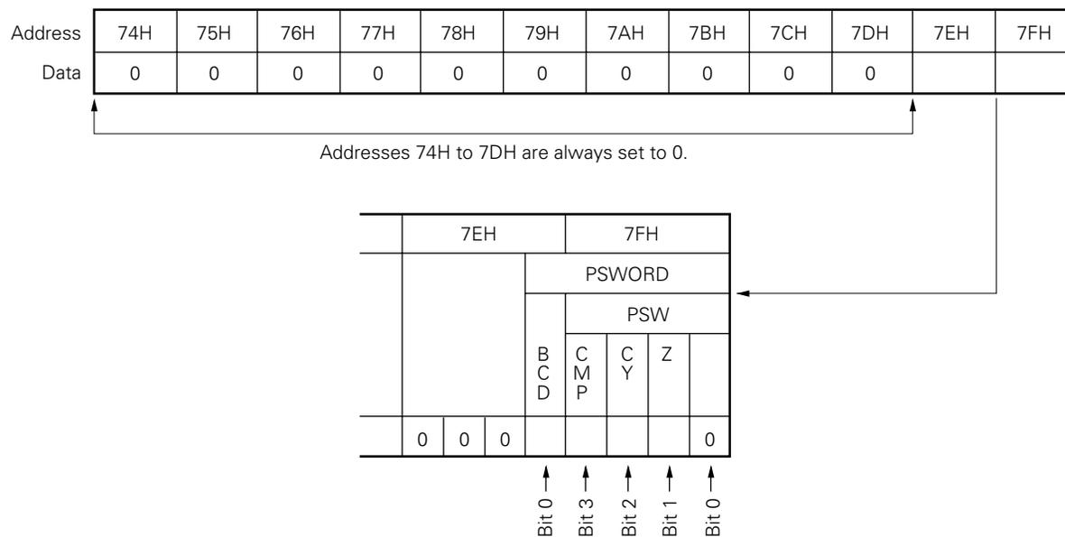
All four bits at address 7FH (PSW) and bit 0 at address 7EH are assigned to the program status word.
