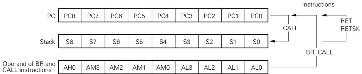
In Fig. 2-1, AH<sub>n</sub>, AM<sub>n</sub>, and AL<sub>n</sub> (0 ≤ n ≤ 3) indicate bit positions in a 16-bit instruction as follows:
