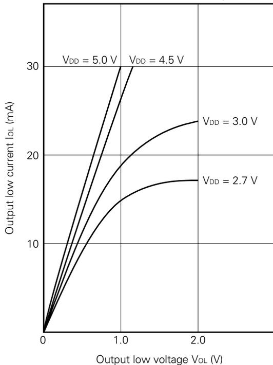
**Caution** The absolute maximum rating of the current is 30 mA per pin. The input voltage or output voltage of the P0E<sub>1</sub> pin must not be higher than  $V_D + 0.3\text{ V}$ .
