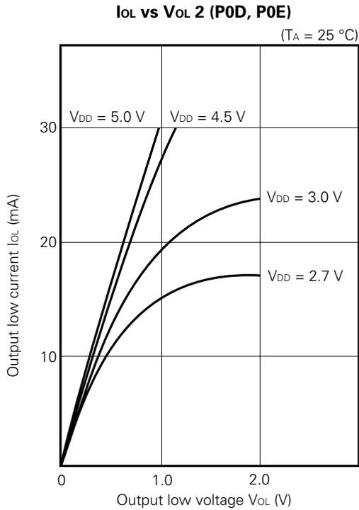
**Caution** The absolute maximum rating of the current is 30 mA per pin. The input voltage or output voltage of the P0E<sub>1</sub> pin must not be higher than V<sub>D</sub> + 0.3 V.
