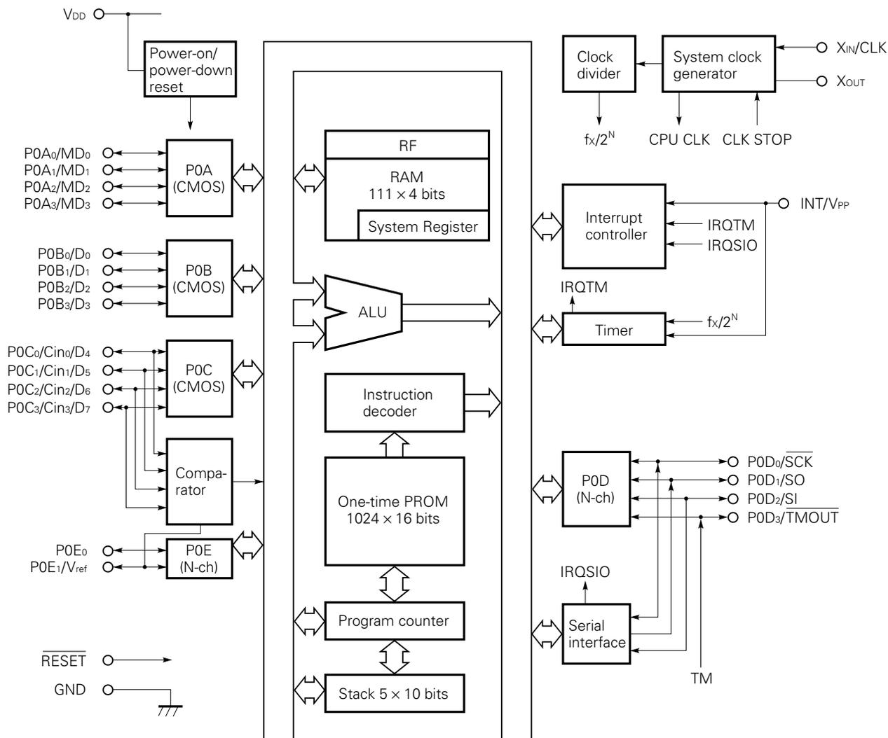
**Remark**The terms CMOS and N-ch in parentheses indicate the output form of the port.
