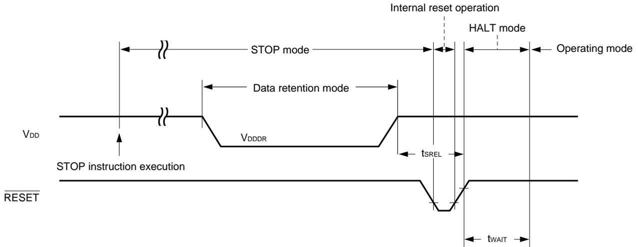
**Data Retention Timing (Standby Release Signal: STOP Mode Release by Interrupt Request Signal)**
