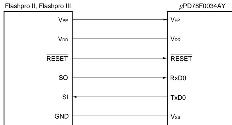
Figure 4-5. Connection of Flashpro II or Flashpro III for Pseudo 3-Wire Serial I/O Mode
