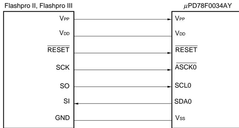
Figure 4-4. Connection of Flashpro II or Flashpro III for UART Mode
