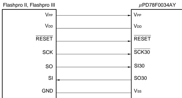
Figure 4-3. Connection of Flashpro II or Flashpro III for I<sup>2</sup>C Bus Mode
