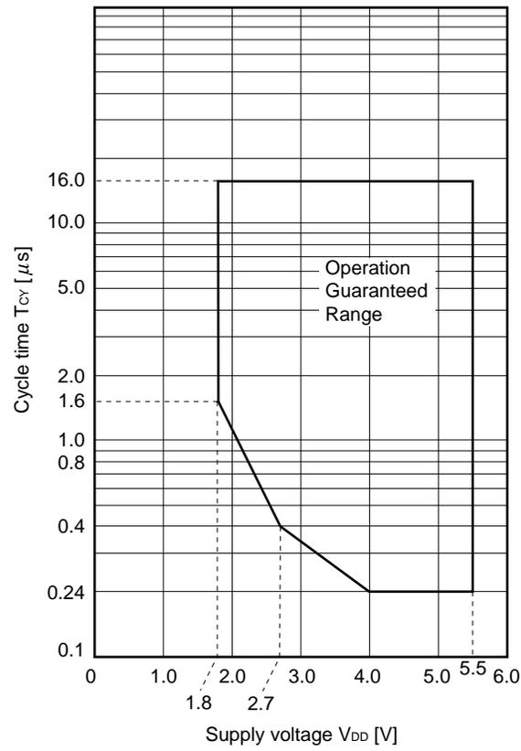
(2) Read/write operation (T<sub>A</sub> = -40 to +85°C, V<sub>DD</sub> = 4.0 to 5.5 V) (1/3)
